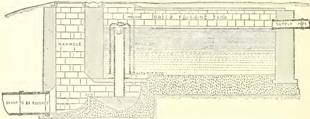
FIG. 4.—Field's Siphon Flush Tank.
