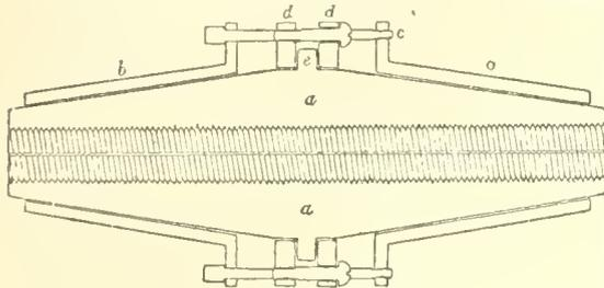
FIG. 1.—Section of grinding nut.
