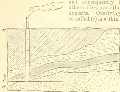
FIG. 2.—Section of Stassfurt Salt-Beds.
