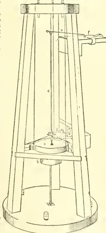
FIG. 1.—Duplex pendulum seismograph.
