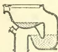
FIG. 16.—Washout Water-Closet.
