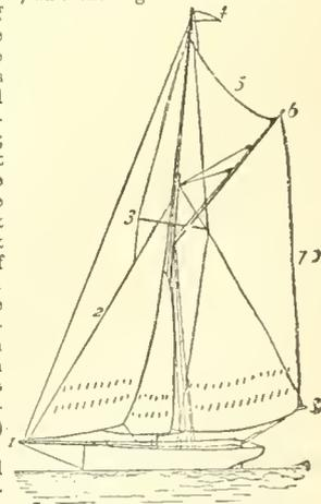
FIG. 37.—Cutter yacht. 1, bowsprit and martingale; 2, jib,—behind it is the fore-sail; 3, cross-trees and top-mast-shroud; 4, pennant, designating the club to which she belongs; 5, gaff-top-sail; 6, peak of gaff, hoisted by peak and throat balyards; 7, main-sail; 8, end of boom and topping-lift.
