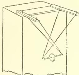
FIG. 9.—Astatic suspension.
