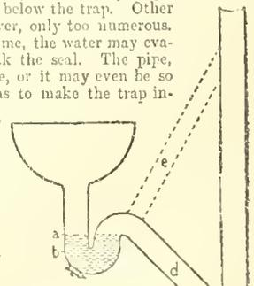
FIG. 5.—Common Water-Trap.
