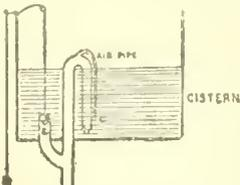
FIG. 18.—Water-Closet Cistern with Siphon Flush.
