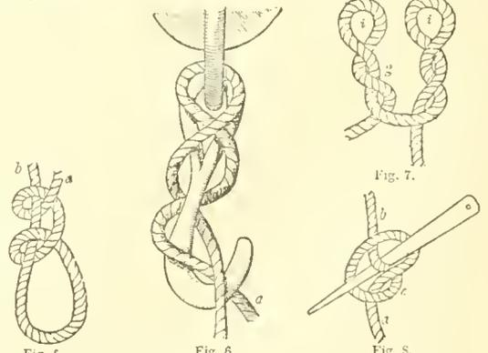
Fig. 5.—Two Half-Hitches.
