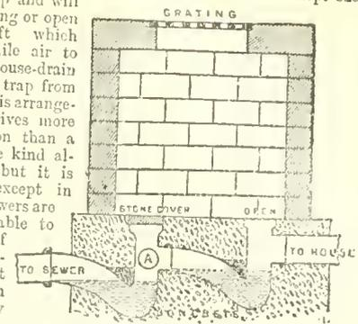
FIG. 8.—Double Disconnecting Trap.
