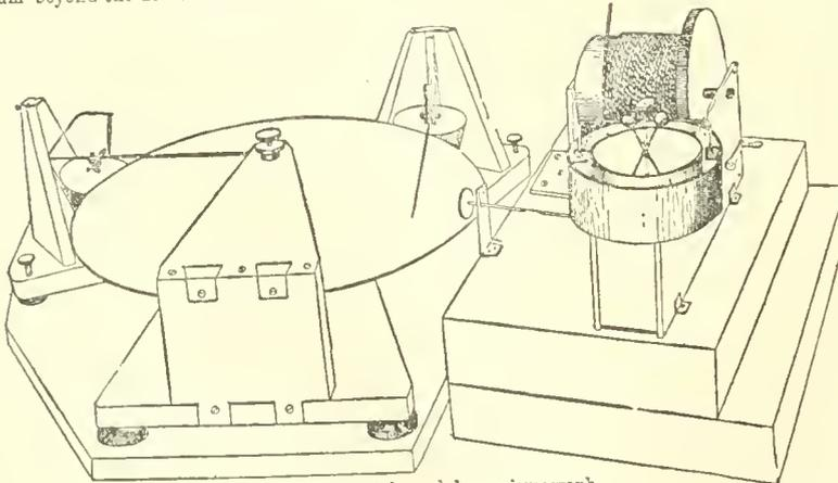
FIG. 5.—Horizontal pendulum seismograph.
