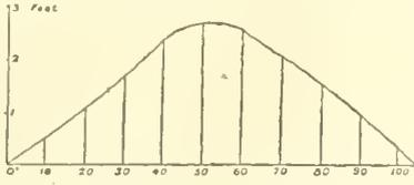
FIG. 5.—Curve of stability of a high-sided ship, having small metacentric height. The vertical line to left shows the various lengths of *d*, and the horizontal line the angles of inclination (in degrees).
