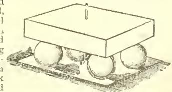
FIG. 4.—Rolling sphere seismograph.
