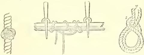
Fig. 16.—Turk's Head. Fig. 17.—Spanish Windlass. Fig. 18.—Slings.
