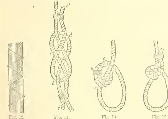
Fig. 12.—Snaking. Fig. 13.—Carrick Bend. Fig. 14.—Insible Clinch. Fig. 15.—Midshipman's Hitch.
