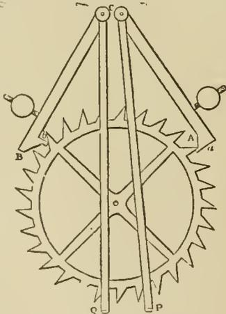
FIG. 10.—Mudge's Gravity Escapement.
