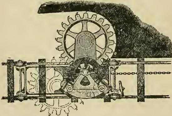
FIG. 14.—Winstanly & Barker's Coal-cutting Machine—Plan.
