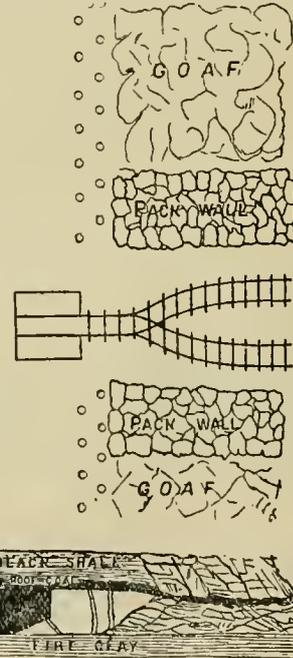
FIG. 12.—Long-wall working-face—Plan and Section.
