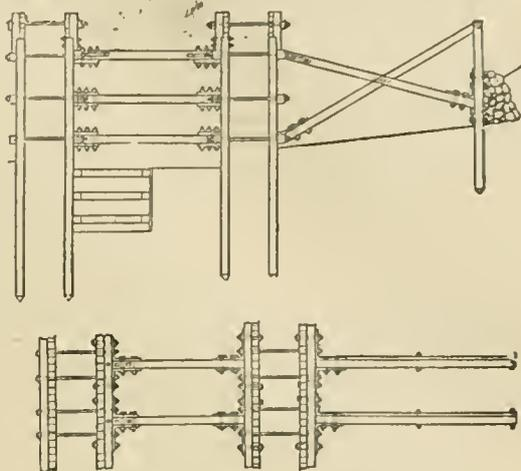
FIG. 2.—Coffer-dam used at Thames Embankment.
