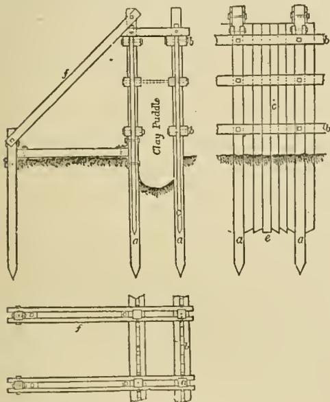
FIG. 1.—Coffer-dam for Soft Bottom.
