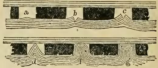
Fig. 7.—"Creeps" in Coal-Mines.
