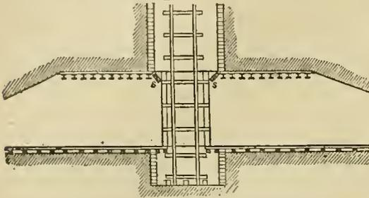
Fig. 5.—Pit eye, Cambois Colliery—Vertical Section.
