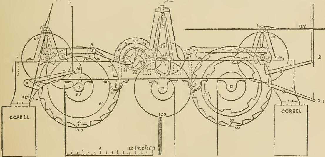
FIG. 22. — Front view of Turret Quarter Clock.
