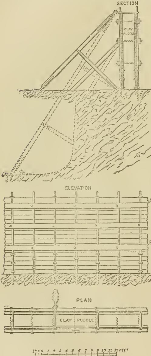
FIG. 3.—Cofferdam for Hard Bottom.
