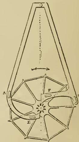
FIG. 11.—Bloxam's Gravity Escapement.
