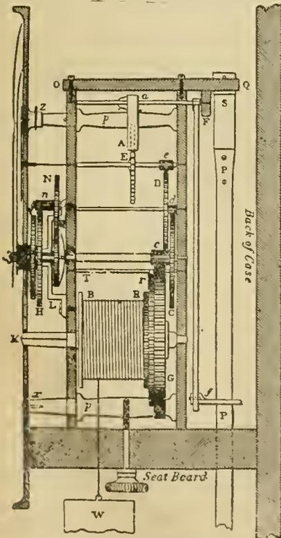
FIG. 1.—Section of House Clock.
