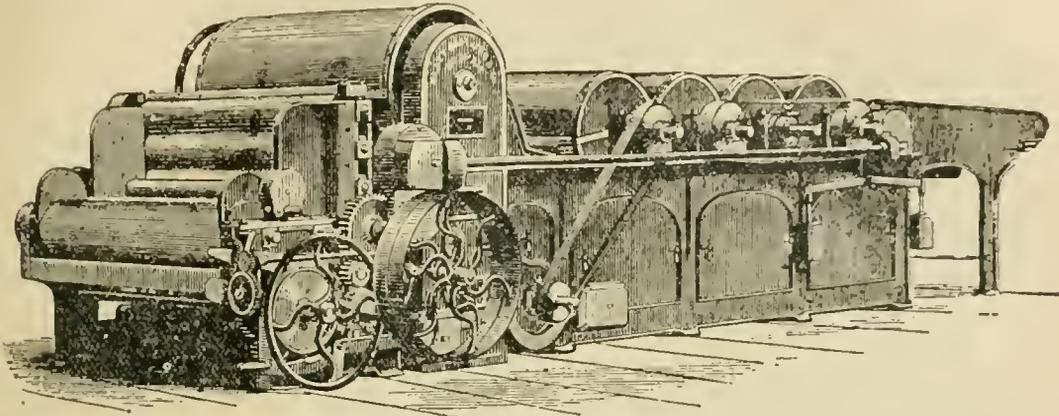
FIG. 3.—Three-cylinder Opener, Beater, and Lap Machine
