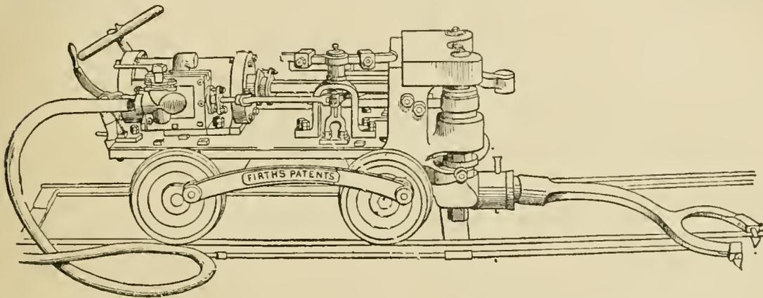
FIG. 13.—Firth's Coal-cutting Machine.
