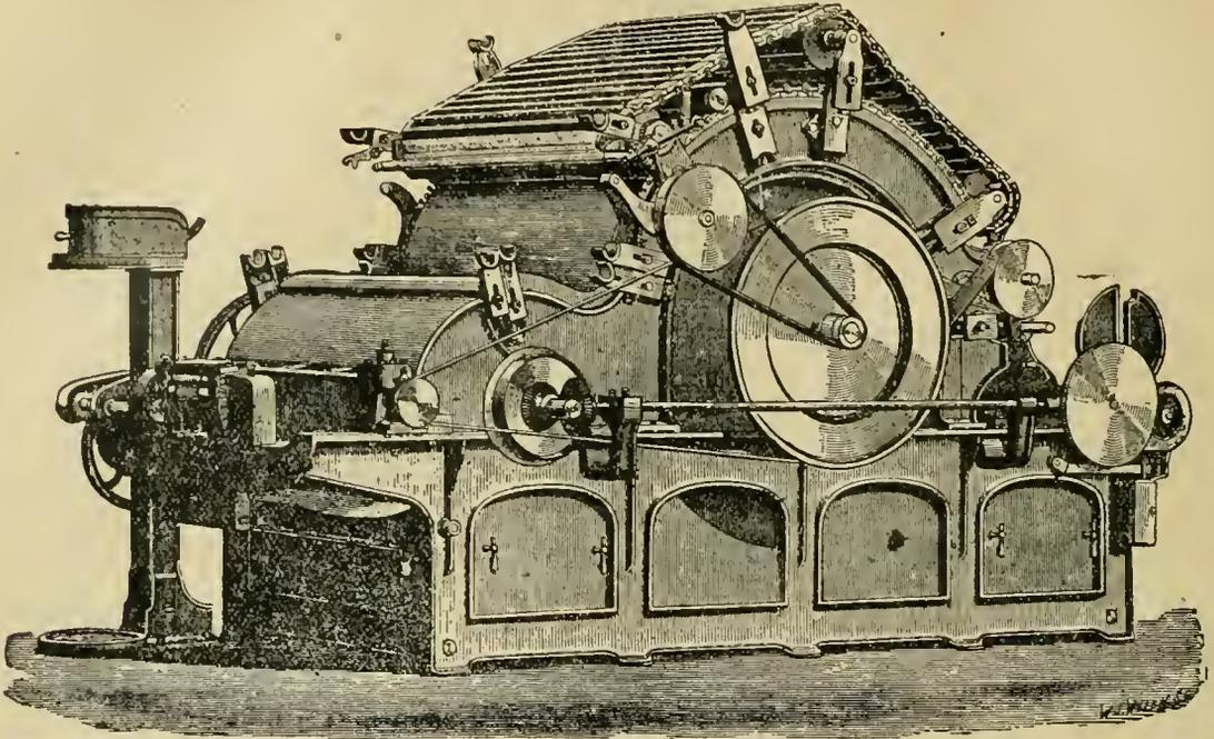
FIG. 5.—Self-stripping Flat Carding Machine.
