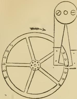
FIG. 6.—Pin-Wheel Escapement.
