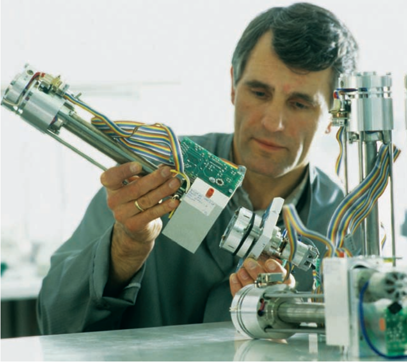
An environmental engineer assembles a sensor used to measure gaseous emissions. Maximilian Stock Ltd./Photo Researchers, Inc.
