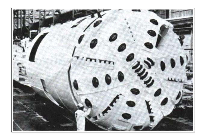
This is a \$13 million tunnel boring machine (TBM) used for tunneling at the Nevada Test Site. (Remember that Area 51 is part of the test site.) Many other types of TBMs are used by many government agencies, including the 'nuclear powered TBM' [NTBM] that melts solid rock and leaves behind glass-like walls.
