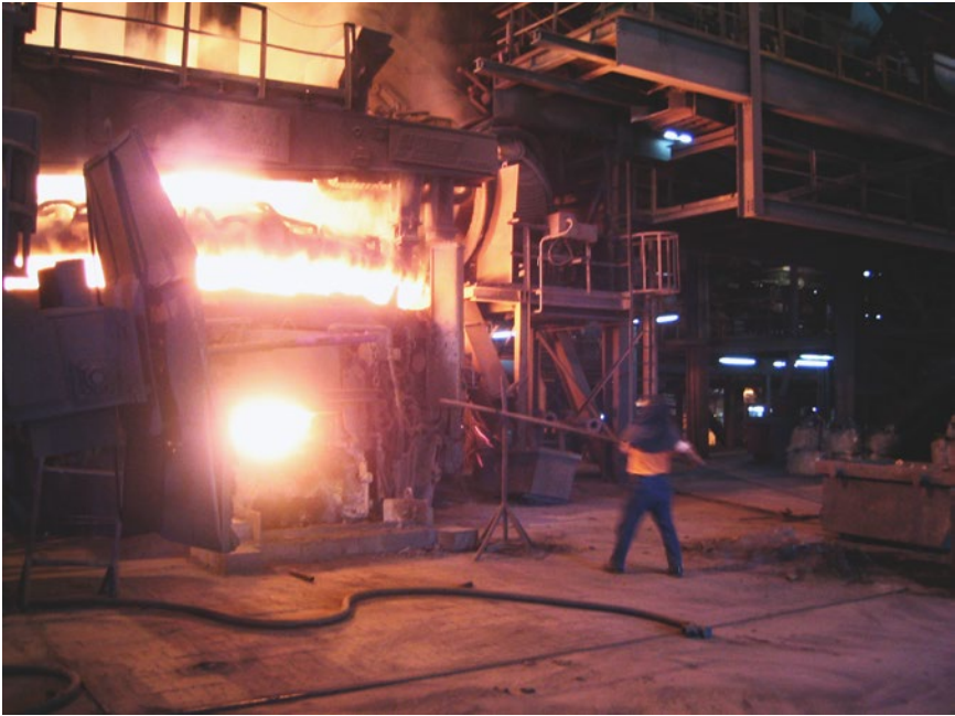
Figure 6.3. A contract worker operating the furnace door of an electric arc furnace at Krakatau Steel.
