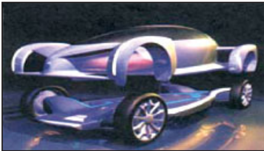
Wireless steering controls, fuel cell “skateboard” mean more flexible body design
