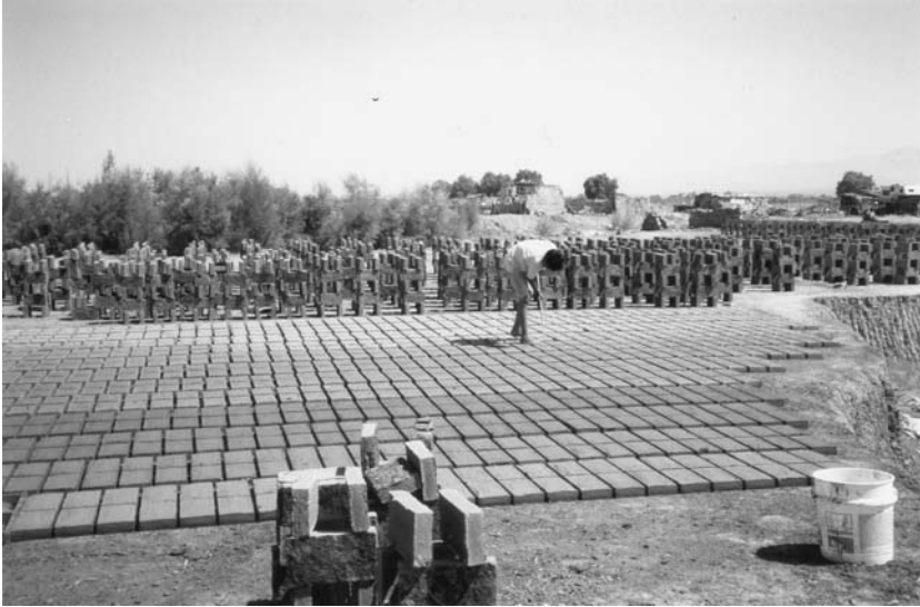
Plate 8. Removing the rough edges from the unfired bricks.
