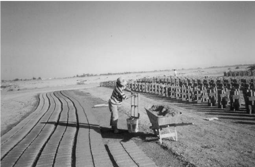
Plates 6 and 7. Molding the bricks with a four-brick mold.
