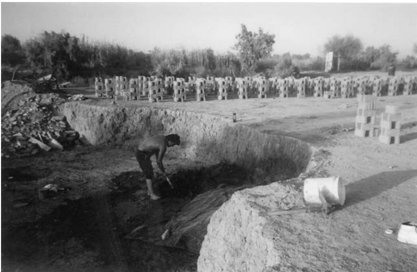
Plates 4 and 5. Digging the clay, prior to mixing with water.
