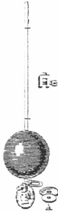
Figure 7.3 Boyle's "hydrometer" – originally for coinage. The illustration features an instrument used to detect counterfeit coins of the realm. Originally designed to monitor guineas, the apparatus can be adapted for lighter coins by adding the circular plates, A, which are made of lead
