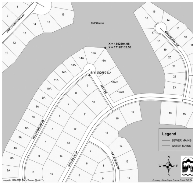
Figure 2 Detail of Corpus Christi Digital GIS/LIS Cadastral Base Map Showing Lot Boundaries and Coordinates in NAD 83 State Plane
