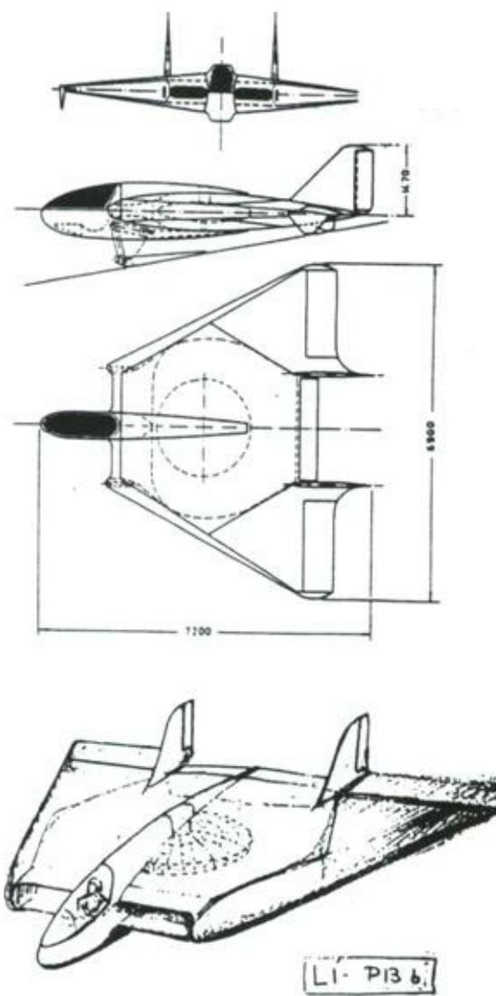
The large air intakes for the ramjets and the disk-shaped combustion chamber are clearly evident. Wind tunnel trials soon showed the advantages of the pure delta shape for supersonic flight, however, and Lippisch produced his final design for the P13b, the final design for which is described in a U.S. intelligence summary for April, 1945:
