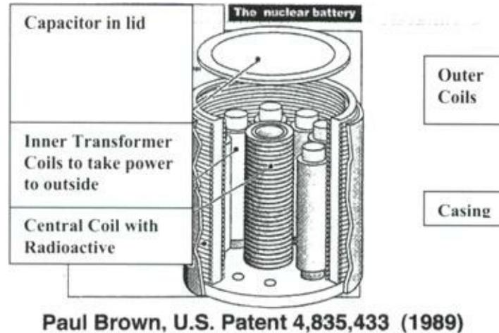
Note the principle of interior and exterior coils, with the central coil, as in the Bell, being stimulated by a radioactive material. The coils also imply that rotation was involved in Brown's thinking from the outset.
