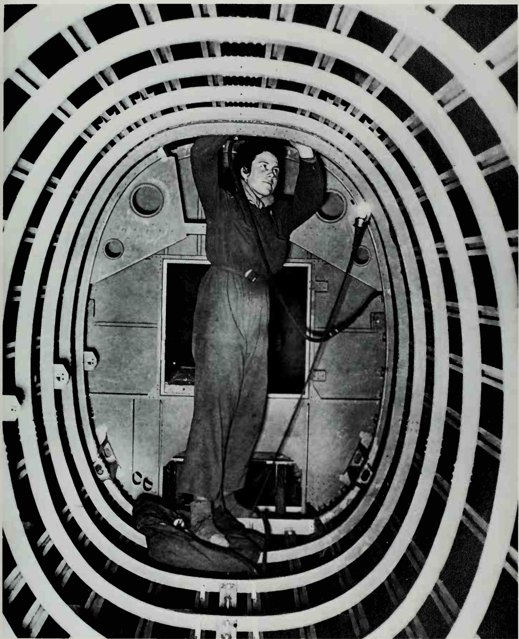
Inside the uncompleted fuselage of a Luftwaffe bomber, a woman aircraft worker balances on a protective pad as she rivets a member into place overhead.
