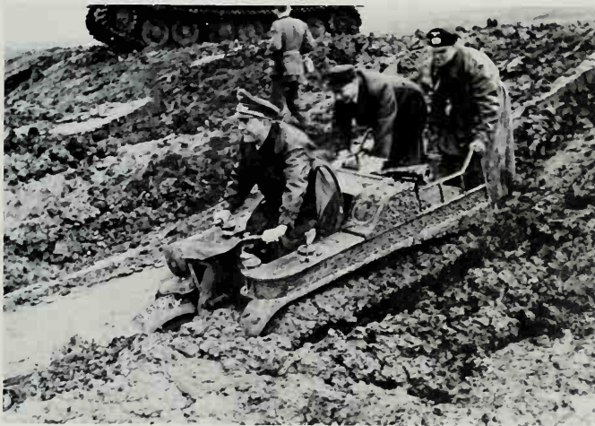
Like youngsters testing a new toy, Production Minister Albert Speer and two aides drive down a muddy slope on a hybrid tracked motorcycle developed in 1943. Speer subordinated Germany's consumer needs to the production of war matériel—in this case a vehicle to overcome "General Mud" on the Russian front.
