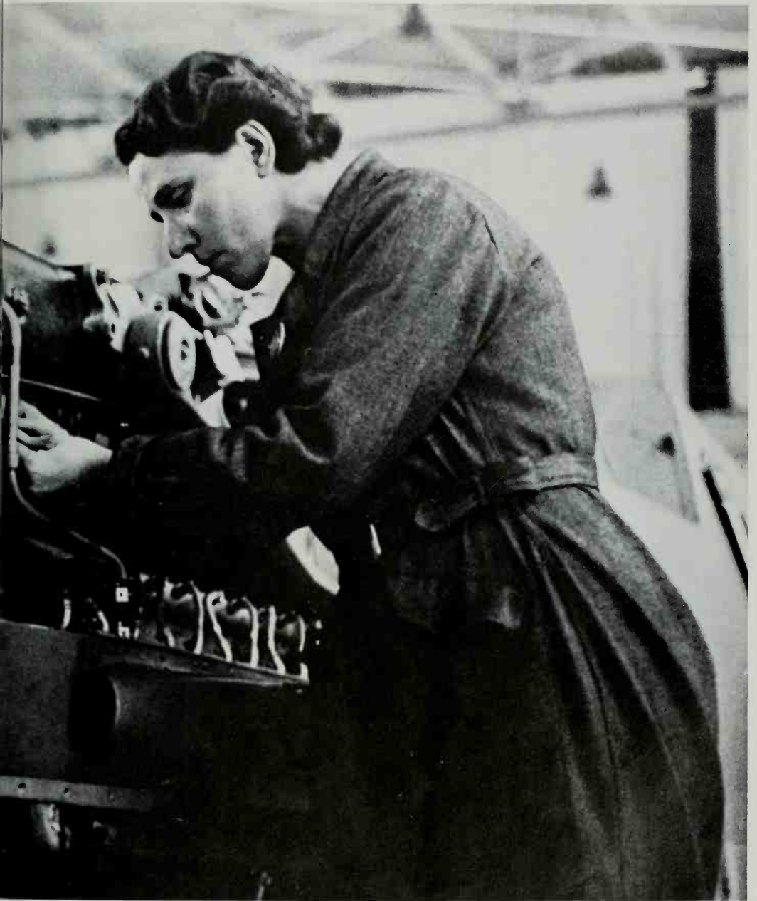
A woman aircraft worker wires the ignition system of a new Messerschmitt-109 fighter plane. German women proved to be adept at such intricate jobs.
