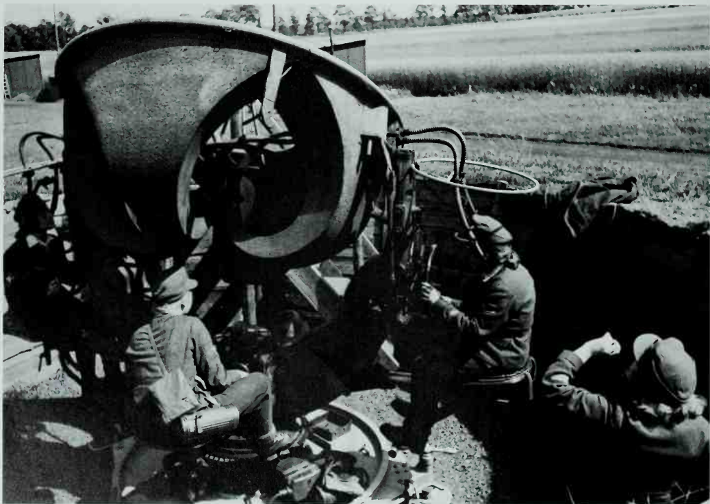
Wearing earphones that are wired to a bowl-shaped sound detector, two women antiaircraft helpers listen for enemy planes while a soldier coaches them.
