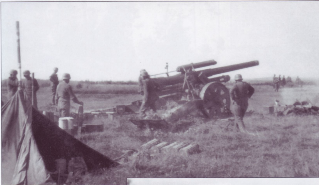
This 15cm howitzer is in full recoil, while an ammunition handler to the rear stands by with a projectile for the next shot. Beside him are propellant cartridge containers. To the right are wicker projectile containers, which artillerymen called a "Koffer" (suitcase). A four-man tent has been constructed using four Zeltbahn shelter-quarters, with a red-and white-striped aiming stake used as the center pole.
