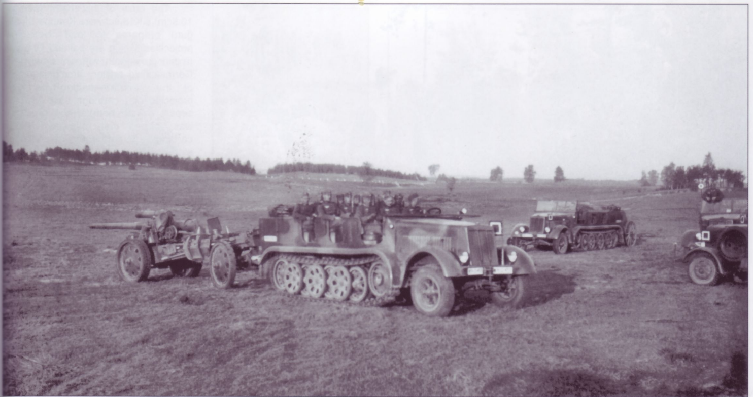
Sd.Kfz. 7 halftracks towing 10cm guns prepare to move out. This appears to be a training scene owing to the neatness of the uniforms and lack of additional equipment. There are also rifle targets lined up on the ridge in the background. This photograph is very likely from the pre-war period since the halftracks are in the three-tone "Buntfarbenanstrich" camouflage scheme of Nr.17 Erdgelb, Nr.18 Braun and Nr.28 Grün, plus they lack the Notek black-out driving head-lamp, which was generally not seen in use until after the French Campaign. One of the halftracks is towing an ammunition caisson of the type used by horse-drawn artillery units.
