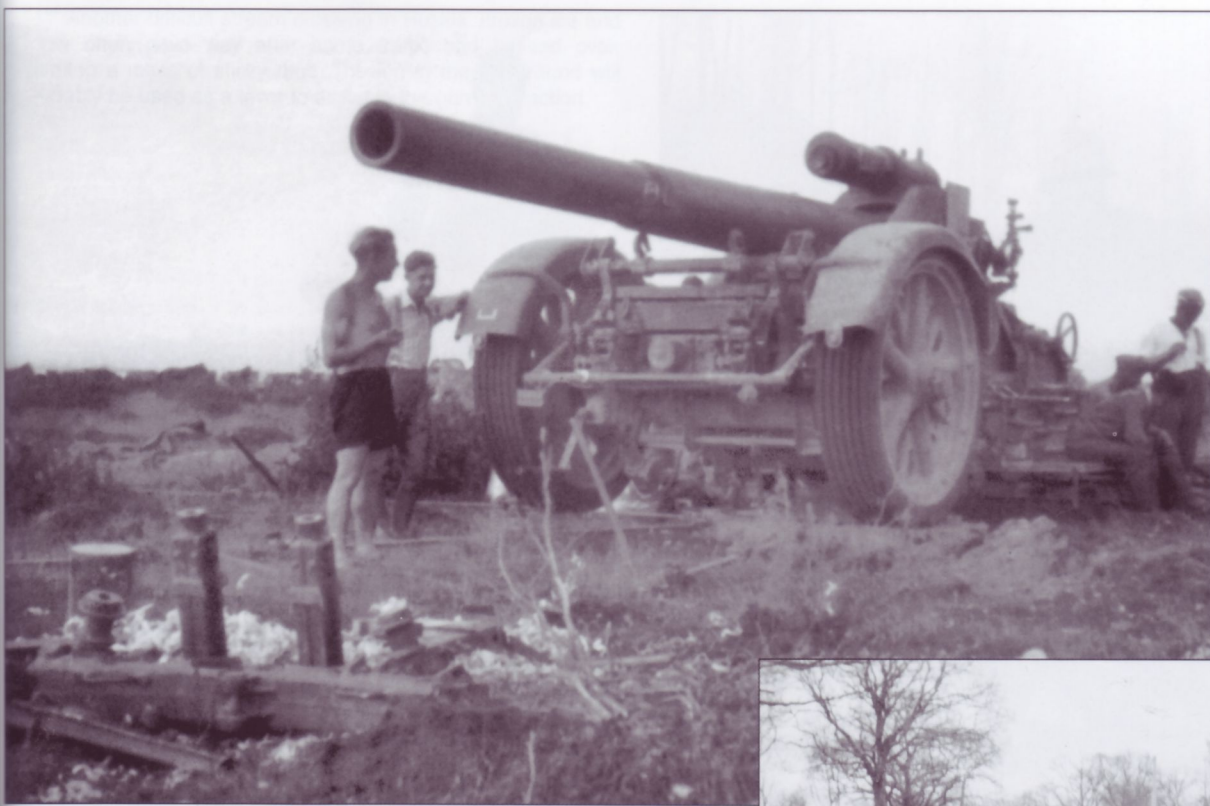
A 21cm Mrs18 heavy mortar in firing position. This same carriage was used for the 17cm s.K18 gun. In the foreground is what appears to be the burned remains of a Soviet artillery piece.
