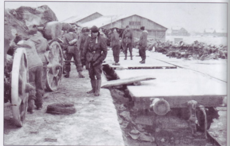
Crews prepare to load their howitzers and limbers on to flatcars. The crews themselves were expected to perform the labor and secure the guns with rope, chains, and wood blocks. When one considers the number of moves any division made, this laborious evolution became routine. Note the piles of debris to the upper right indicating the rail-yard had been heavily bombed at one time, probably by the Germans, who later repaired it for their own use.
