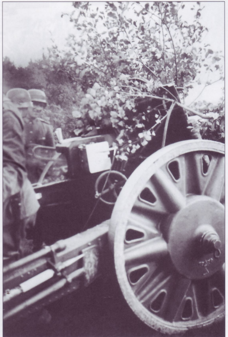
This 10.5cm le.FH18 has just ejected a spent cartridge. The wheel, as found on most German artillery pieces, consisted of a heavy duty cast steel hub with a solid rubber rim. This type of tire allowed relatively high-speed towing by a motorized vehicle. Unlike inflatable tires, they had the advantage of being immune to blowouts and light shell fragmentation damage. The hard rubber rim would wear down, but could be replaced. Note the spade and handspike fastened to the gun's trails, as well as the foundry casting symbols on the wheel hub.
