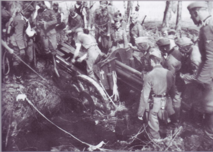
Battery personnel are assembled to manhandle a 10.5cm howitzer out of a stream, where a hastily-constructed timber bridge has collapsed. The six horses were unable to pull the gun, which weighed 5,589-pounds in travel order, out of the steep-banked stream. Note the pick fastened to the gun shield.
