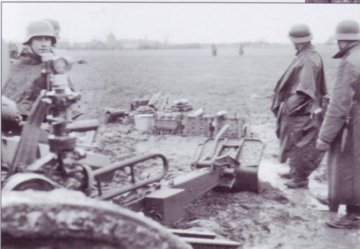
A view of the ready ammunition station behind the gun. Here the propellant cartridges were issued in metal-lined wicker containers rather than wooden boxes. The Geschützführer to the left looks to the rear at two figures in the distance, that are relaying firing orders. Though blurred, to the left of the gun tube, near the wheel, can be seen an M32 panoramic telescope, the standard sight used on many German artillery pieces.
