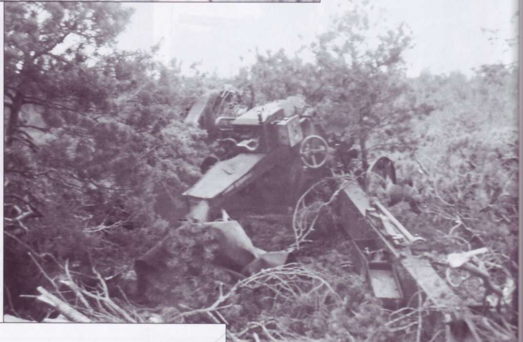
This 10.5cm le.FH18 leichte Feld Haubitze (light field howitzer) has been demolished by Soviet counter-battery fire, with the shield and right wheel being destroyed. Note that the horizontal sliding breech block is in the open position. The gun was positioned among fir saplings and further camouflaged by cut saplings stacked around it.
