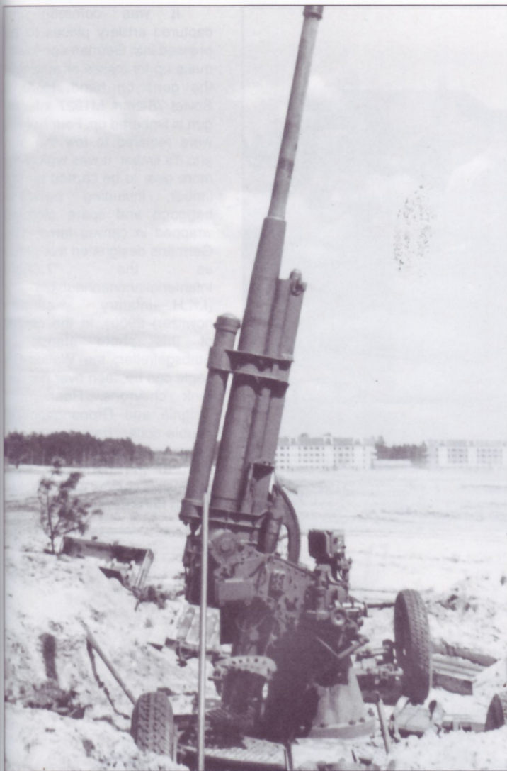
This is a Soviet 85mm M1939 anti-aircraft gun overrun by the Polizei-Division outside of Leningrad. Though obviously prepared to engage aircraft, the Soviets often employed them in the anti-tank role in the same manner the Germans used the "88". The 85mm AA guns was sometime pressed into German service where it was known as the 8.5cm FlaK M39(r). The "(r)" identified a captured piece of equipment as being "russisch", or of Russian-origin. Some were re-bored to use German 8.8cm ammunition. In that case the designation was 8.5/8.8cm FlaK M39(r).
