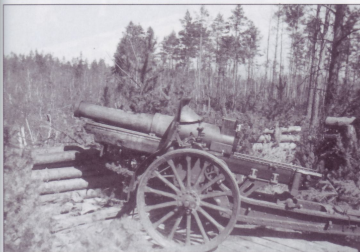
The French Schneider 155mm C mle.1917 howitzer was sometimes issued as a substitute for the 15cm heavy howitzer. The Germans called it the "15.5cm s.FH414(f)". They also used it as a coast defense weapon, not as an anti-ship gun, but to shell the assault troops. It fired a 96.16-pound shell out to 12,362 yards. The howitzer has been positioned on a plank platform behind a two-layer log breastwork.
