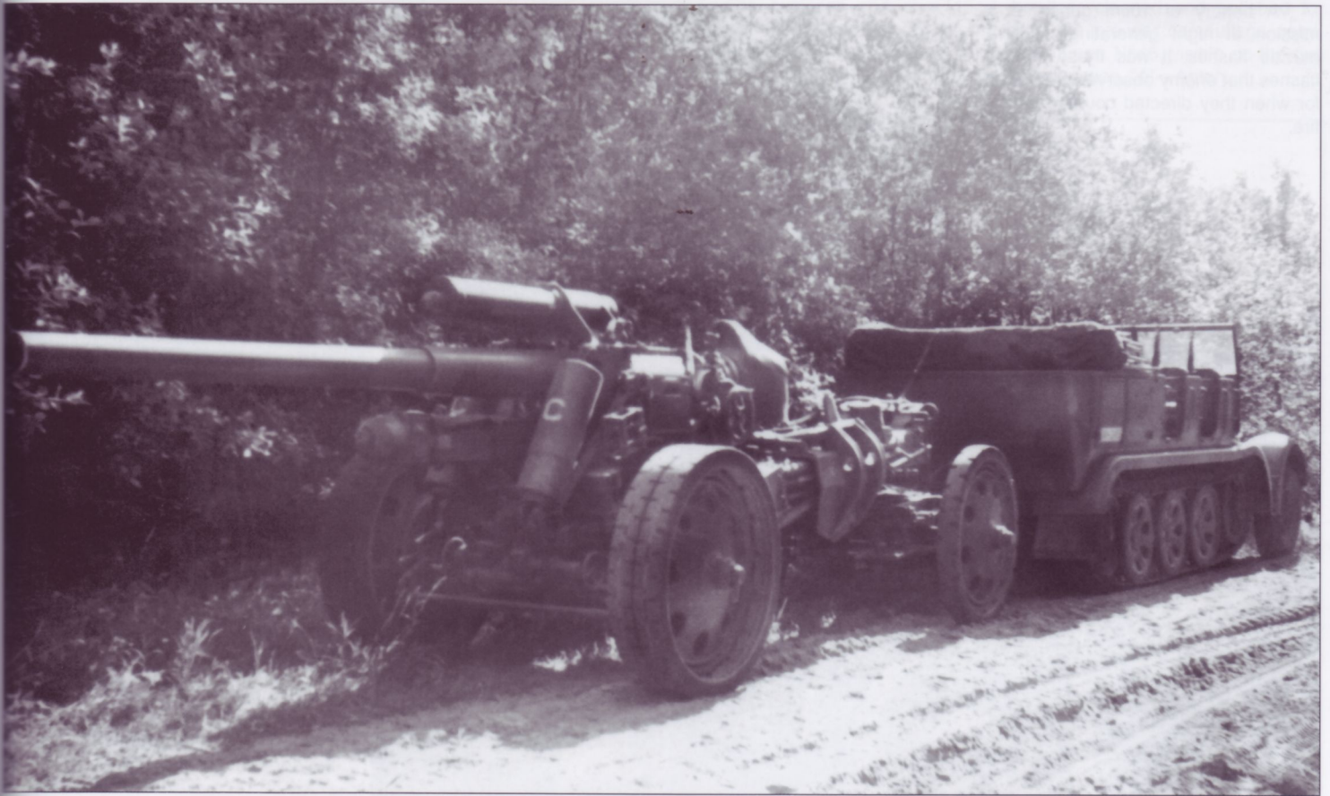
This view of a 10cm s.K18 depicts it in the travel position. The gun tube appears shorter as it has been retracted past the "recoil" position to lessen the overall length of the piece and shift the weight more towards the limber for a better balance of the load. The white "C" on the hydro-pneumatic equilibrator cylinders identifies the gun within the battery. They were designated by the German phonetic letters—Anton, Bertha, Caesar, and Dora—used for transmitting alphabetical letters by radio and telephone so they could be understood through static or a poor connection. The type of cast steel wheel with rubber rims, pictured here, was intended for motorized towing. The prime-mover is an early Kfz.7; it could also tow the 15cm s.FH, 10cm s.K and 8.8cm FlaK.
