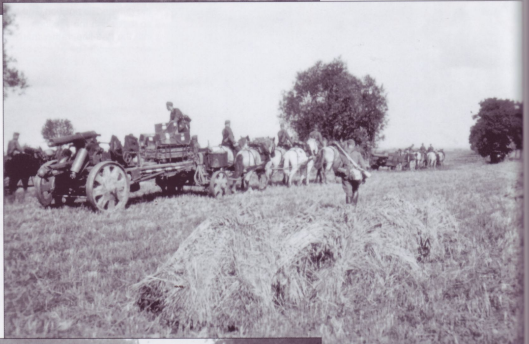
When drawn by horses, the 15cm howitzer was broken down into two loads, each drawn by six horses. Here the carriage and mounting are seen, with equipment secured to the gun's trails. The gun tube and breech was carried on a special four-wheel transport wagon, seen to the right.
