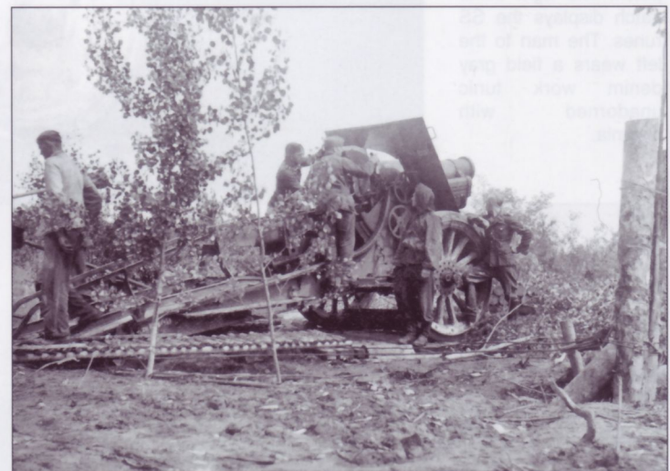
Another view of a French 155mm C mle.1917, also known as the 15.5cm s.FH414(f). A few saplings have been stuck into the ground as minimal camouflage to include one wired to the "dead-man" post to the right. To this is fastened block-and-tackle by which the gun is pulled back into a protected bunker. The foot ramps on either side provide the loaders with firm footing as they carry the 96.16-pound projectiles to the piece.
