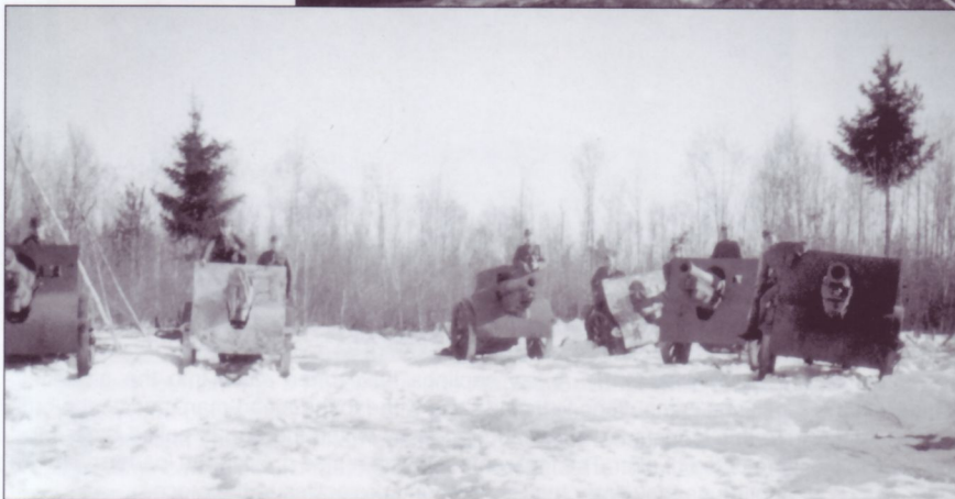
This collection of weapons are mostly French-made Schneider 105mm mle.1919 mountain guns formerly used by the Yugoslavians. The Germans employed them as the 10.5cm leichte Gebirgshaubitze (I.Geb.H.—light mountain howitzer) 329(j). It could be broken down into eight pack-horse loads; the gun tube could be disassembled into two parts to ensure that no single load was too heavy. Some of these guns have had whitewash applied for winter camouflage.
