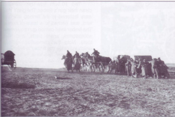
Despite the power of six horses, this crew has to provide an assist as the team strains to drag this gun and limber up a gradual slope. Iron-shod horse hooves had difficulty gaining a purchase on icy snow. This is a 10.5cm le.FH16 light field howitzer, a World War I weapon adopted in 1916. It was widely used before the war, but relegated to second-line units when the more modern 10.5cm le.FH18 was fielded.
