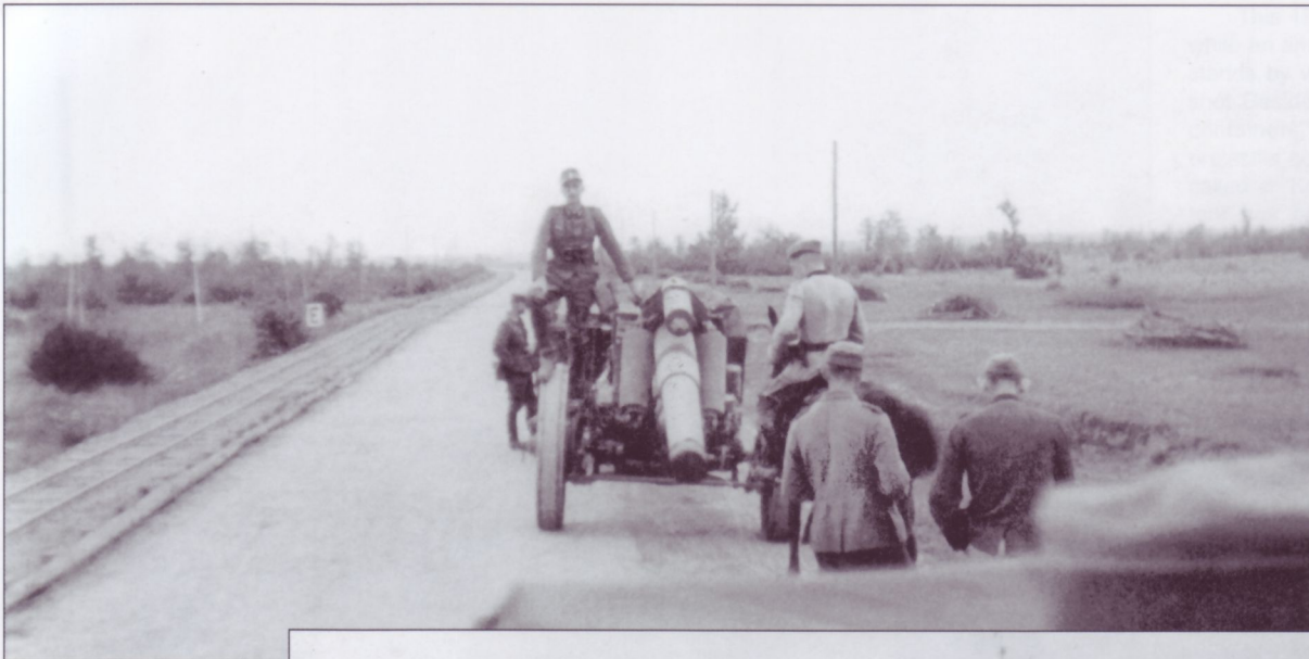
A 15cm howitzer assembled for firing, probably during training; note the sign next to the tracks. A team of horses could tow the fully assembled piece short distances for positioning. A narrow-gauge railroad, laid by the Germans to haul supplies, parallels the well-maintained road.
