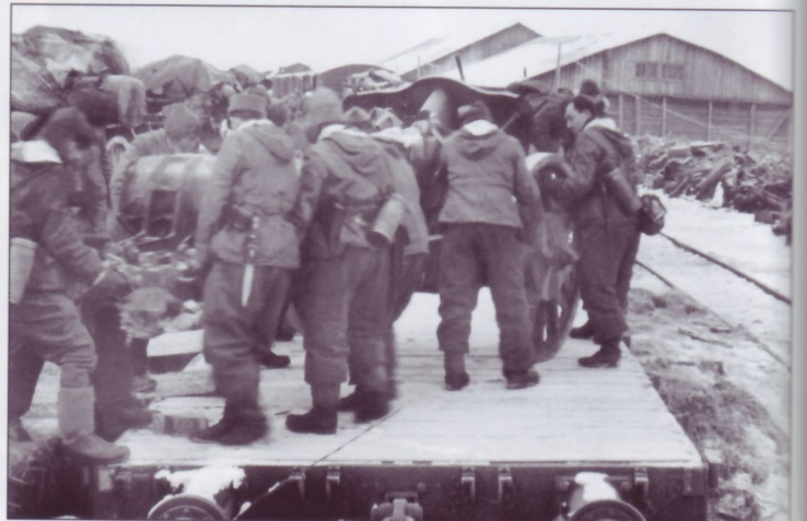
Crews prepare to load their howitzers and limbers on to flatcars. The crews themselves were expected to perform the labor and secure the guns with rope, chains, and wood blocks. When one considers the number of moves any division made, this laborious evolution became routine. Note the piles of debris to the upper right indicating the rail-yard had been heavily bombed at one time, probably by the Germans, who later repaired it for their own use.
