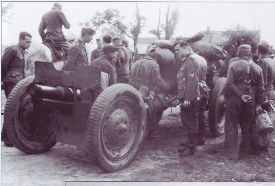
A similarly camouflaged Soviet 122mm M1938 howitzer has been impressed into German service as the 12.2cm s.FH396(r). This was one of the best and most reliable Soviet artillery pieces of the war, being highly valued by the Germans. It had a range of 12,909 yards. The man to the right is an SS-Rottenführer, identified by the double chevrons and left collar patch. The right collar patch displays the SS runes. The man to the left wears a field gray denim work tunic unadorned with insignia.
