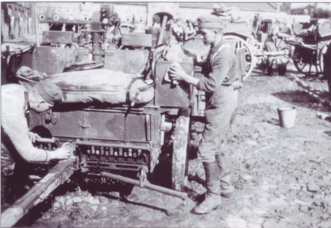
Two 10.5cm howitzer crewmen clean their gun's limber. The gun's trails were fastened to the limber, which, in turn, was hitched to a team of horses. The limber itself carried gun equipment, accessories, spare parts, and hand tools. Note the camouflage pattern which indicates the limber is finished in the early war two-tone scheme of Dunkelgrau Nr.46 and Dunkelbraun Nr.45.
