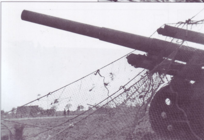
A 15cm s.FH18 schwere Feld Haubitze (heavy field howitzer) sits beneath a hastily erected camouflage net. The bare net, unadorned by vegetation or garnishing, provided little concealment. Besides concealing the weapon, camouflage nets also served to deny the enemy the ability to identify what type of artillery piece occupied the position or if the position was actually occupied by a real gun.
