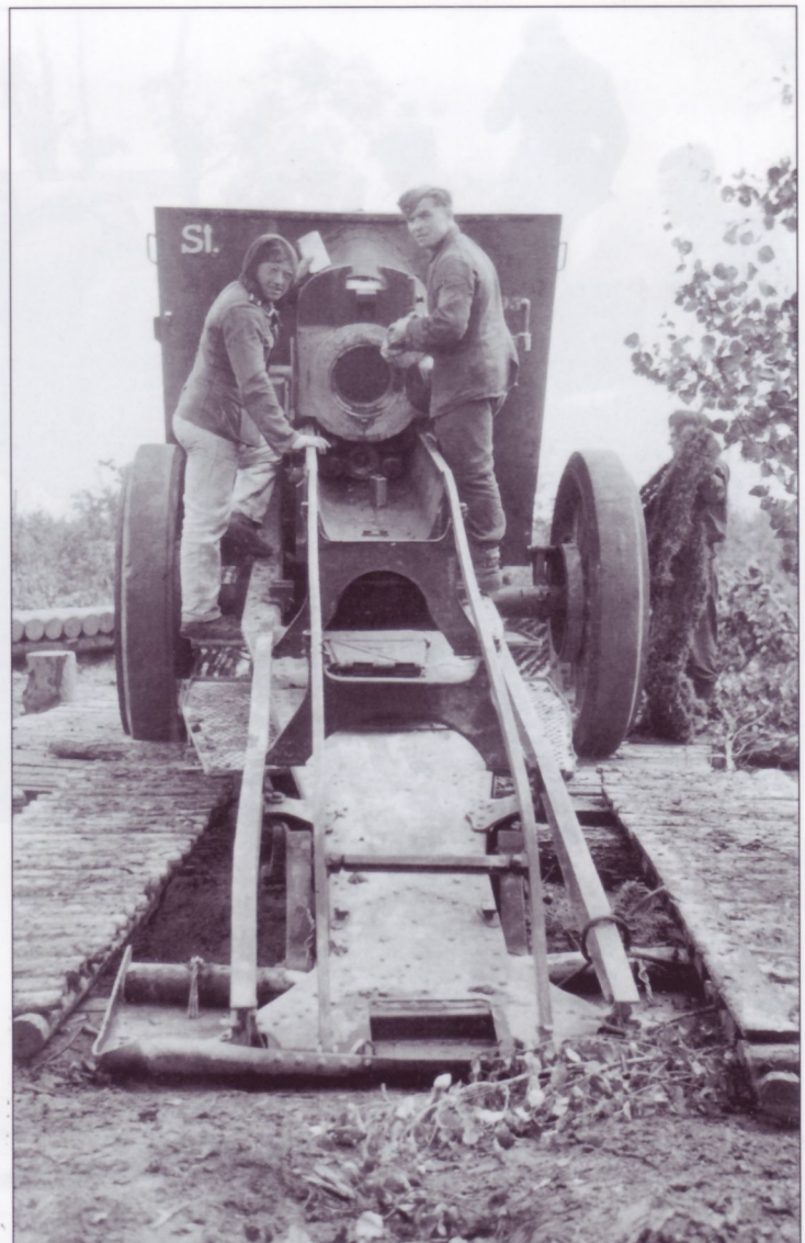
A small number of captured French Schneider 220mm mle.1916 breech-loading mortars were used during the Leningrad siege. The Germans designated it as a 22cm Mrs531(f). The mortar could lob a 221-pound shell 11,000 yards at a rate of two rounds per minute. The meaning of the legend "St." is unknown; it was used for a number of abbreviations in the Wehrmacht, but none apply to a gun designation.
