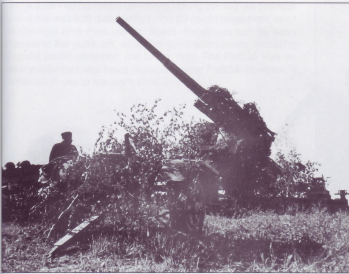
An 8.8cm FlaK18 of SS-Flak-Abteilung 4, assigned to 4.SS-Polizei-Panzer Grenadier-Division is positioned for the air-defense role. The gun and its limbers have been lightly camouflaged with cut foliage to help conceal their silhouettes from low flying aircraft. Crews were provided with camouflage nets, but these were time consuming to erect and dismantle, so they were often not used during short halts.
