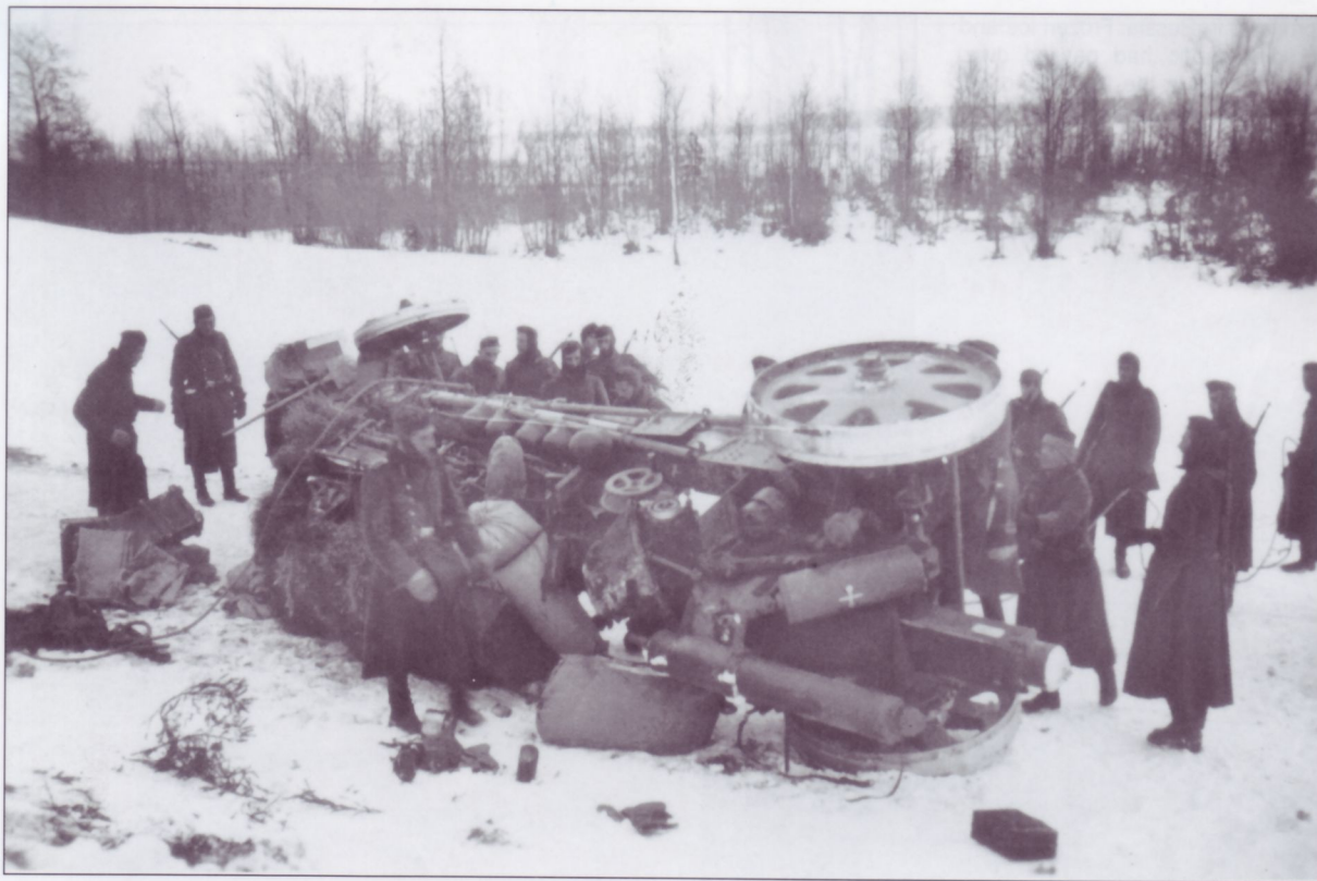
The heavy carriage of a 15cm howitzer has slid off the ice-covered road. The steel-rimmed wheels offered no traction on ice or wet hard-surfaced roads. Among the scattered gun equipment are bales of hay for the draft horses. It was essential that fodder be carried for the horses in the winter when no grazing grass was available. Note the crew's helmets fastened to the piece's trail.
