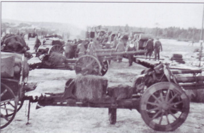
A battery of 10.5cm le.FH18 howitzers are lined up to load aboard railroad flat cars during one of the Polizei-Division's many moves. The howitzers are attached to their limbers, with bales of hay on the gun trails for the draft horses. Note the difference in wheel types and the fact that the second howitzer is the "M" version with a muzzle brake. The guns are painted with light-colored stripes over the Dunkelgrau RAL 7021 base color. The evenly spaced paint dabs on the wheel rims actually detract from the camouflage effect since orderly camouflage patterns attract the eye rather than disrupt the appearance of the piece of equipment.
