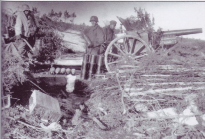
A 10.5cm le.FH16 light field howitzer in a firing position with saplings and brush stacked for concealment. Two seats for crewmen were fitted on the front of the shield either side of the gun tube, on which they rode during travel. Projectiles and their packing tubes are seen beside the gun. The le.FH16 had a feeble range of 1,203 yards as opposed to the le.FH18's 11,678 yards.
