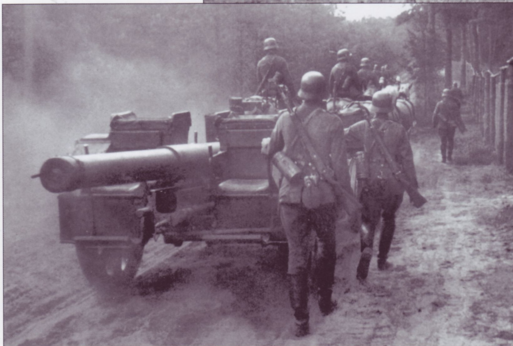
Here the gun tube and breech of the 15cm howitzer are seen on its transport wagon traveling through a Russian forest. The transport wagon used the same wheels as the gun carriage. The crewmen are wearing only minimal equipment with the rest being carried aboard limbers, caissons, and the transport wagon. The men on foot carry their gas mask containers in the normal dismounted troops' position while those on horseback wear theirs as specified for mounted soldiers. Although the transport wagon was fitted with seats, crewmen often preferred to walk as the un-sprung wagon was uncomfortable, while the less the horses had to haul, the better for all concerned.
