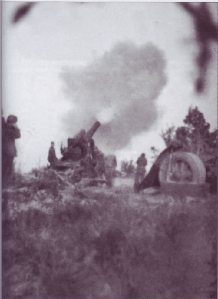
This massive weapon is a 21cm Mrs18 heavy mortar. It was not assigned to divisional artillery, but to army- or corps-level artillery formations, which could be tasked to support a division. It could toss 266.8-pound high explosive or 285.3-pound anti-concrete projectiles up to approximately 18,300 yards. Note the huge limber wheel to the right, partly concealed by saplings.
