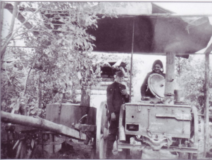
On the right is a field kitchen, which could simultaneously cook 29-gallons of soup or stew, as well as brew 16-gallons of coffee. Four insulated 12.5-quart food containers were provided to carry the food to gun positions. To fuel the cook fires, the unit could burn coal, coke, charcoal briquettes, or wood. To the left is a captured Soviet mobile cooking cauldron.
