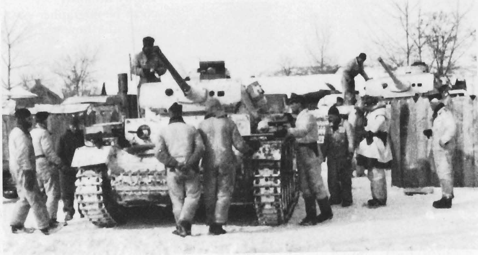
The Armored Regiment was equipped in part with Panzer III tanks. These were superior to the Panzer IV in speed and handling, but too weakly armed with their 5 cm KWK guns.
