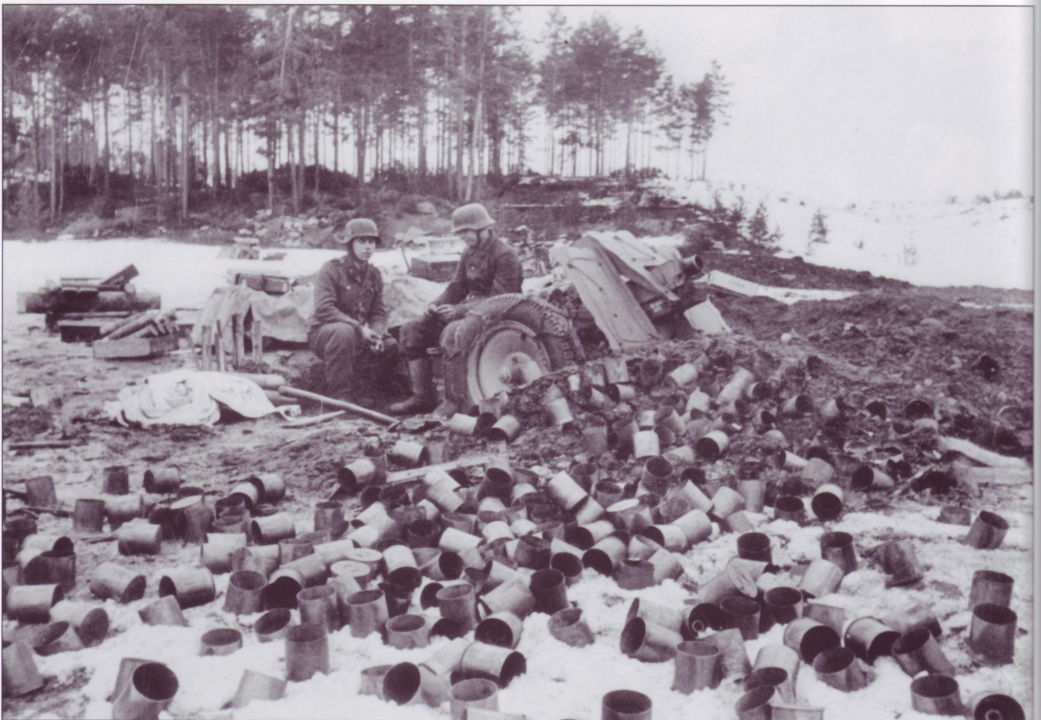
The crew of this 7.5cm I.G.18 light infantry gun have obviously been busy supporting its parent unit in the Narva area in April of 1944. Two such guns were usually attached to each battalion of an infantry regiment for direct and indirect fire support. Ice chains are secured to the tires for better traction in slippery conditions, while the wire on the shield is for attaching foliage.
