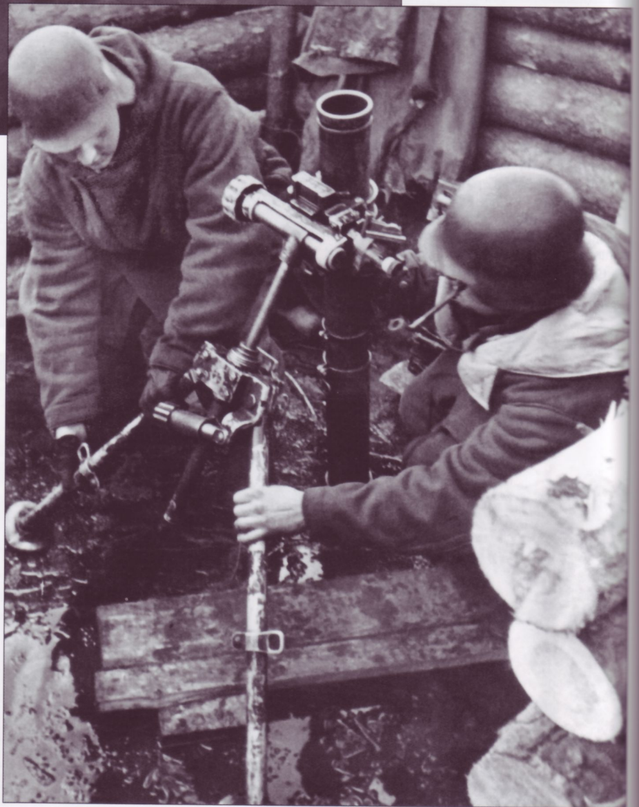
Another weapon equipping the battalion machine gun company was the 8cm m.Gw.34 medium mortar (mittlerer Granatwerfer). Six armed the company's mortar platoon. The Russians used the similar 82mm mortar, which could fire German 8cm ammunition (actually 81mm), but the Germans could not fire Russian ammunition. The Germans did use large numbers of captured Russian mortars though and fired their own and Russian ammunition. This Granatwerferneist appears to be above ground or just partly below ground and has an open front allowing a clear field of fire. Even if above ground the pine logs provided some protection for light shell fragments.
