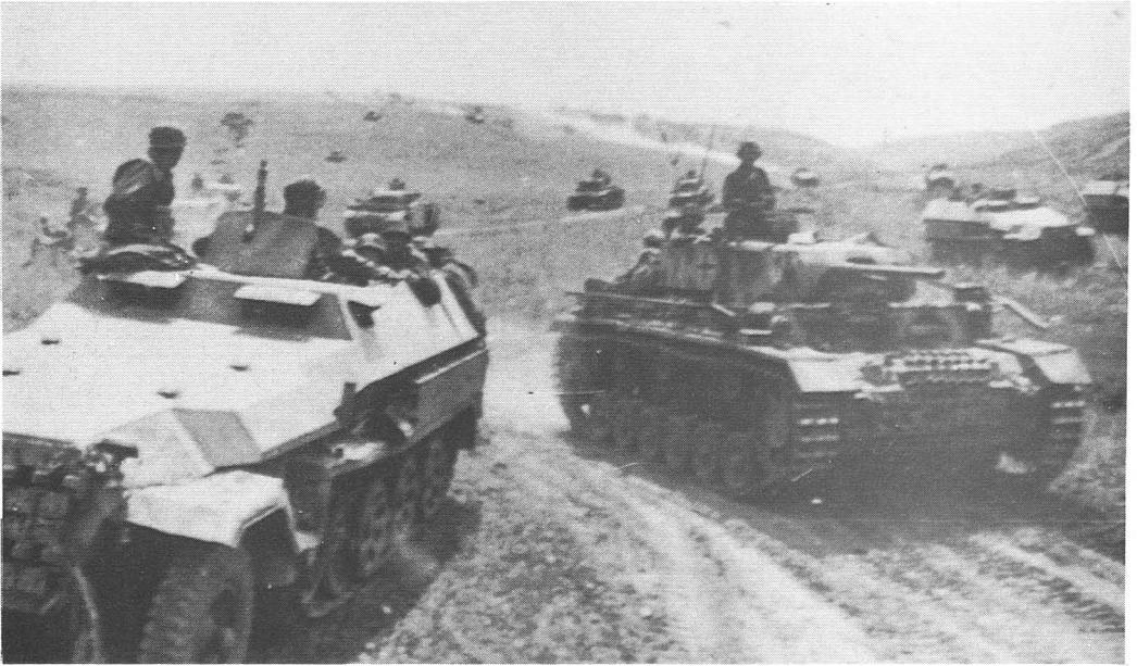
Above SdKfz 251 (foreground) which, interestingly, appears to have spare tank track links attached to its bonnet for added armour protection; and PzKpfw III, of the 'Das Reich' Division, during the Battle of Kursk (73/80/40).
