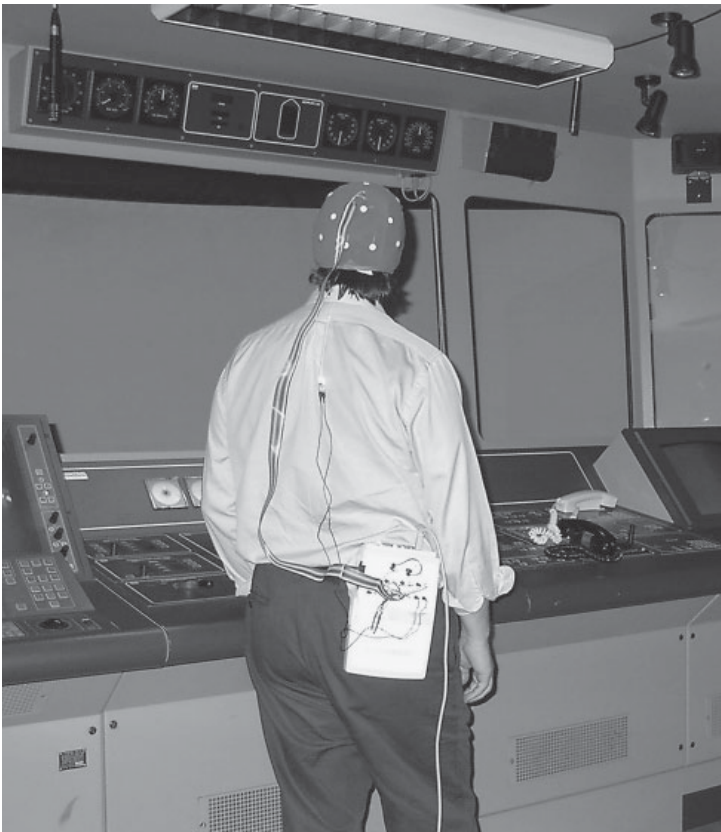
Figure 29.1 The experimental set-up of the electrode cap and the amplifier (fitted in the belt of the participant) in the maritime full mission simulator
