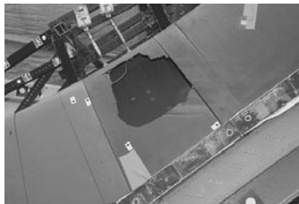
FIGURE 6.8. Breach in Orbiter Wing (CAIB Photo by Rick Stiles 2003; http://www.caib.us/photos/view3ad4.html )
