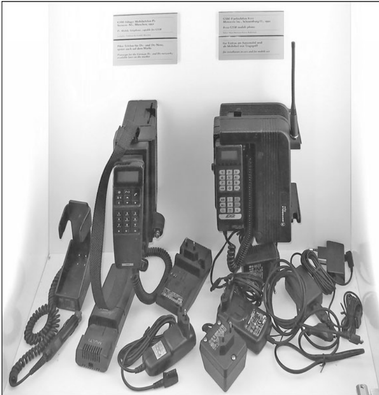
Figure 2.3 The first phones capable of text messages—two 2G GSM phones with chargers and base stations. Photo courtesy of Clemens Pfeiffer via Wikimedia Creative Commons License 2.5, a freely licensed media repository.
