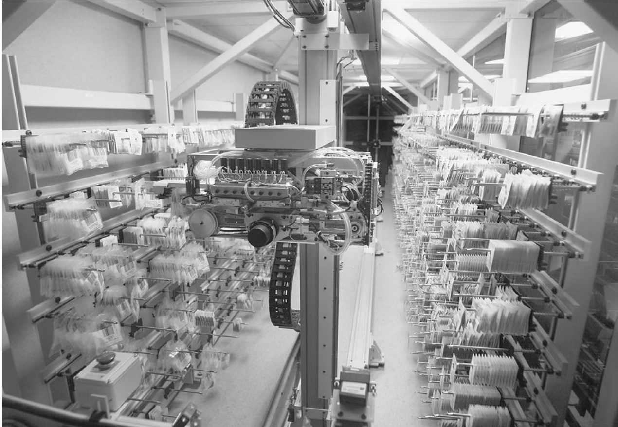
Robby the Robotic Pharmacist, Hackensack University Medical Center. Following data entered in the hospital's computer system, Robby uses his "arms" to find prescriptions to be given to patients among the sorted medicine packets on the wall. © ED KASHI/CORBIS
