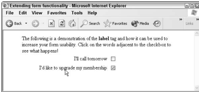
Figure 10-3: By including the label tag, clicking the text next to the check box causes the box to be checked.
