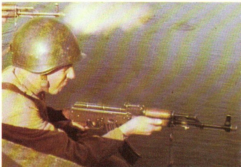
Above: Soviet infantryman fires the 7.62mm AKM assault rifle, a modernisation of the AK 47, in production since 1959. Note the small recess in the side of the receiver, directly over the magazine, and the small muzzle compensator: both are among the features that distinguish it from the AK 47.
