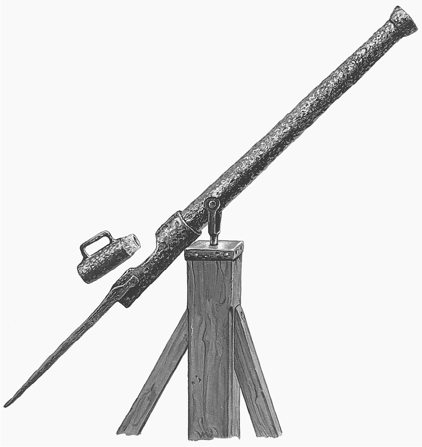
Falconet with breech removed (Courtesy Art-Tech)
