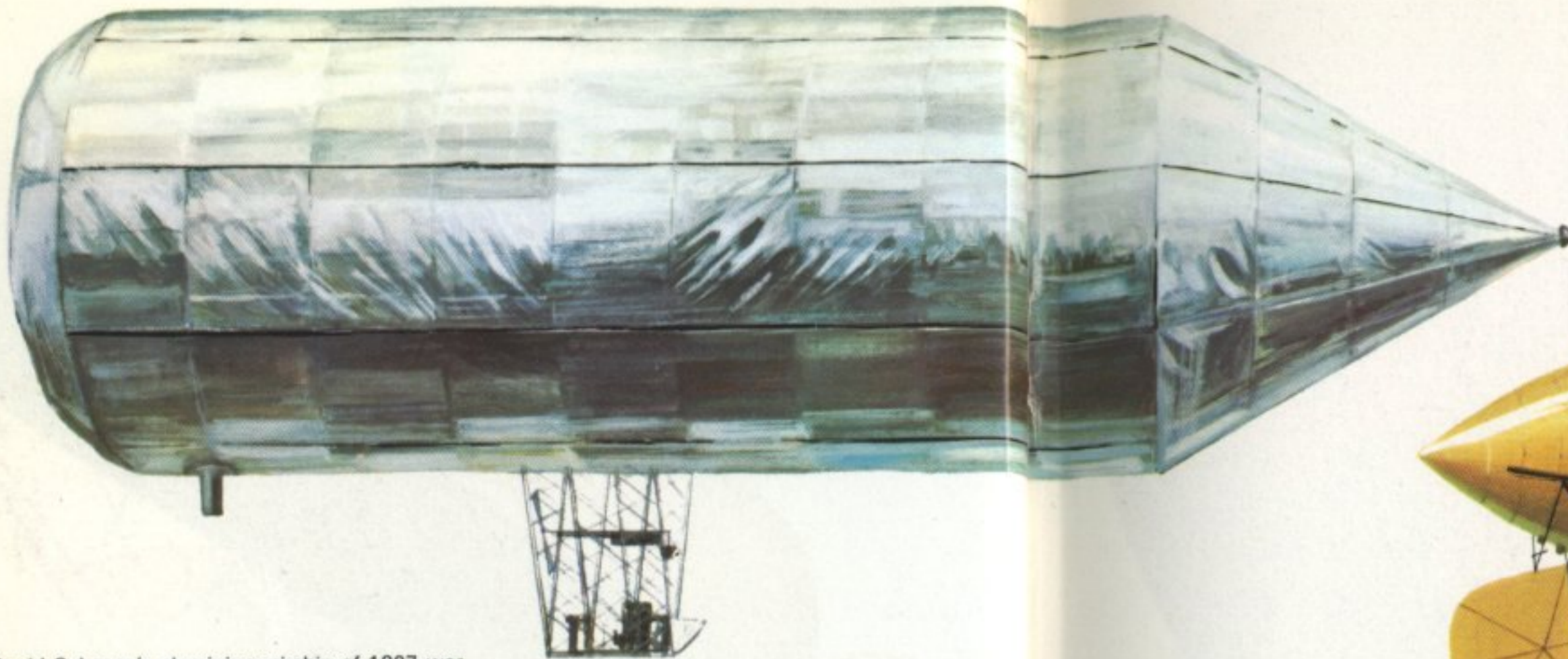
22 David Schwarz's aluminium airship of 1897 was a technical advancement for its day. It was wrecked due to poor handling on its trial trip at Schöneberg near Berlin.
