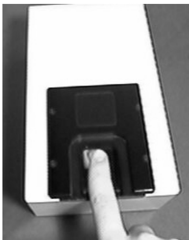
Figure 8.5 FTIR fingerprint scanner manufactured by Digital Biometrics. (From Digital Biometrics, Digital Biometrics Homepage, http://www.digitalbiometrics.com/ . With permission.)
