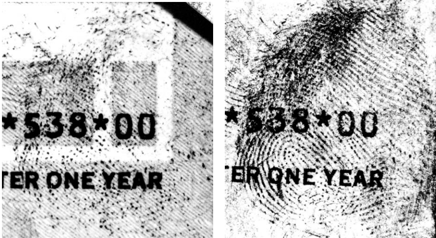
Figure 7.4 Comparison of a ninhydrin print on a forged United States Treasury check before (left) and after Ag-PD treatment (right). Ninhydrin print is enhanced.
