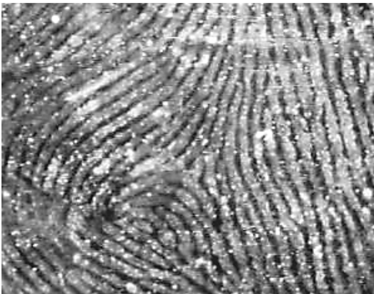
Figure 6.19 Photoluminescence of fingerprint (on aluminum foil) developed by diimide-mediated CdS/generation 3.5 dendrimer treatment (see text).
