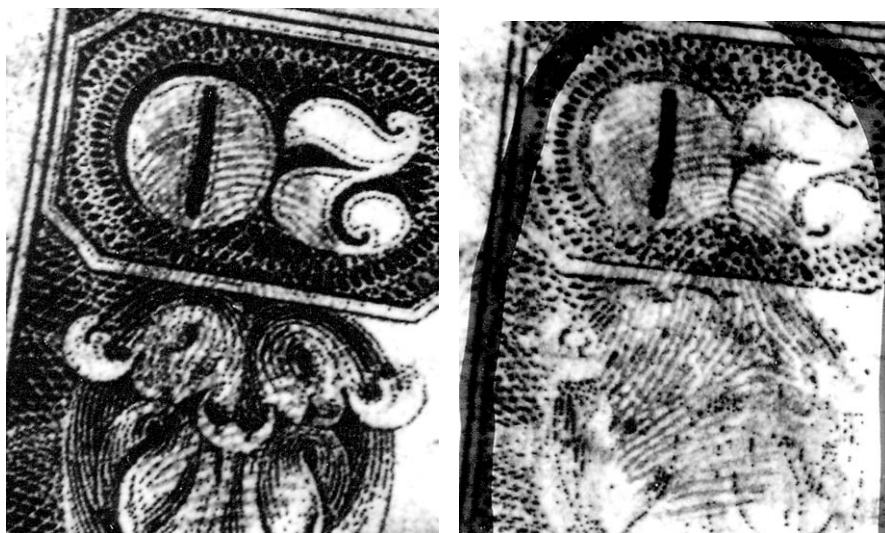
Figure 7.6 Comparison of an Ag-PD print on a counterfeit $20 note before (left) and after hypochlorite bleach treatment (right). Ag-PD print darkens and background lightens.
