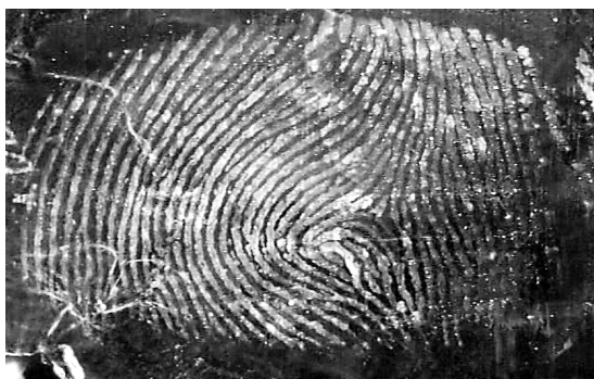
Figure 6.15 Photoluminescence of fingerprint on polyethylene fumed with cyanoacrylate ester and subsequently stained with CdS/generation 4 dendrimer methanol solution.
