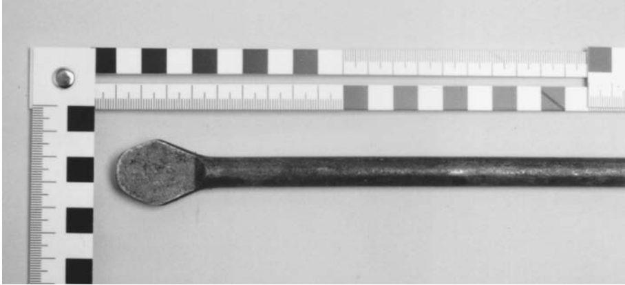
Figure 8.10 The tool that created the pattern in Figure 8.9 . Note the beveled edge where the tool head and shaft come together. This characteristic is clearly visible in the pattern in Figure 8.9 as the elliptical area void of blood. (Photograph courtesy of Jouni Kiviranta, National Bureau of Investigation, Helsinki, Finland.)
