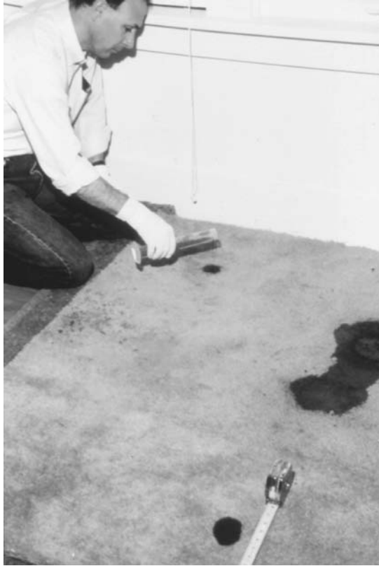
Figure 8.30 The next step is to create a similar-sized stain on a similar surface. Blood is added slowly and the size of the stain created monitored by the analyst. This is done in order to match the general dimensions of the stain in question as closely as possible.
