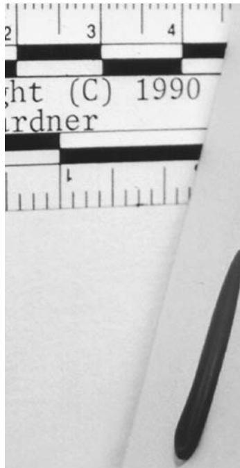
Figure 4.15 Early displacement of a droplet impacting at an acute angle. Note the distinct rim in the leading edge.
