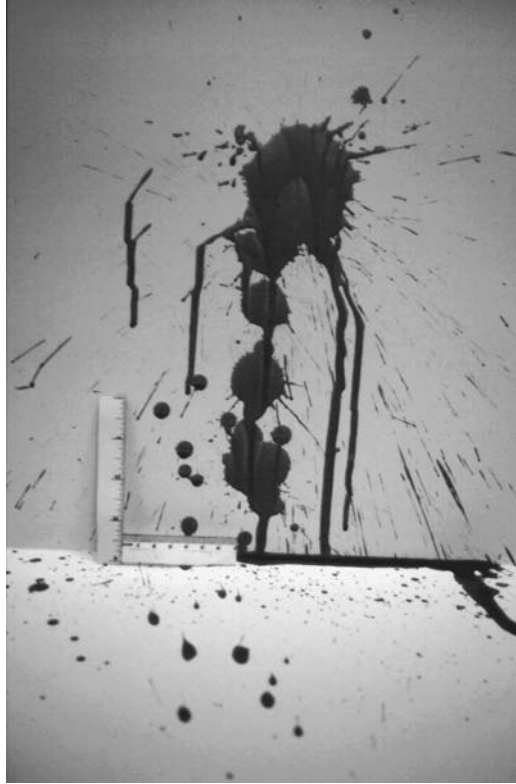
Figure 3.30 A splash pattern. This splash pattern was produced in a laboratory setting by tossing a small volume of blood against the target. Splash patterns tend to have a cohesive look, with little breakup of the blood into smaller stains.
