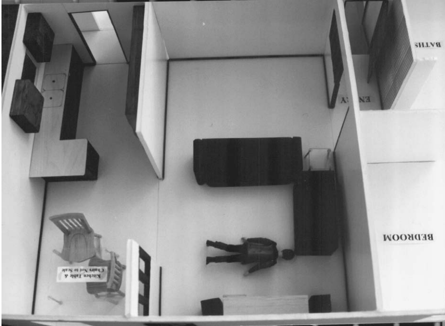
Figure 12.4 The foam core model. Although not used as often due to the availability of software programs, such models are still effective tools.
