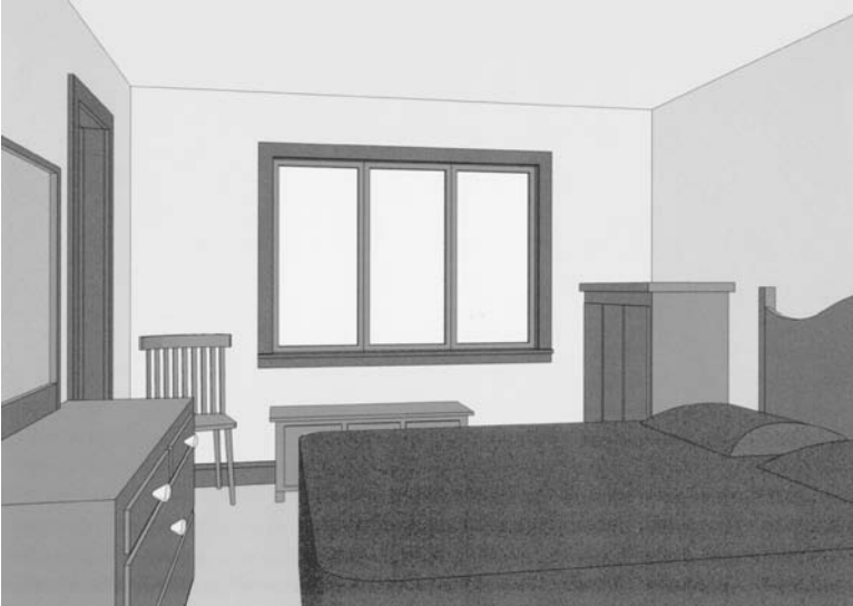
Figure 11.12 These programs allow the placement of a camera to create a view from anywhere within the scene. In this example we show the view across the room from the doorway. The software will usually accommodate whatever view is necessary. The view is then exported as an image (usually a bitmap) and imported into the presentation software.
