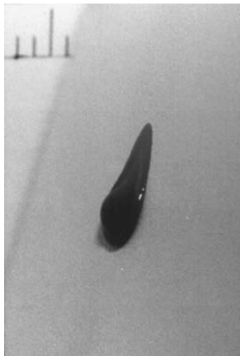
Figure 4.13 Late contact/collapse phase of a droplet impacting at an acute angle. In this photograph about half of the sphere is still intact and evident in the center of the expanding stain. Note that the majority of the blood is being forced into the rim opposite the direction of origin.
