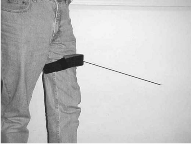
Figure 12.2 A Velcro and foam device in which the trajectory rod is placed and then attached to the body. This allows a more dynamic understanding of how the movement of an individual may affect the alignment of a given trajectory. In this photograph, with the leg straight, the trajectory is slightly downward.
