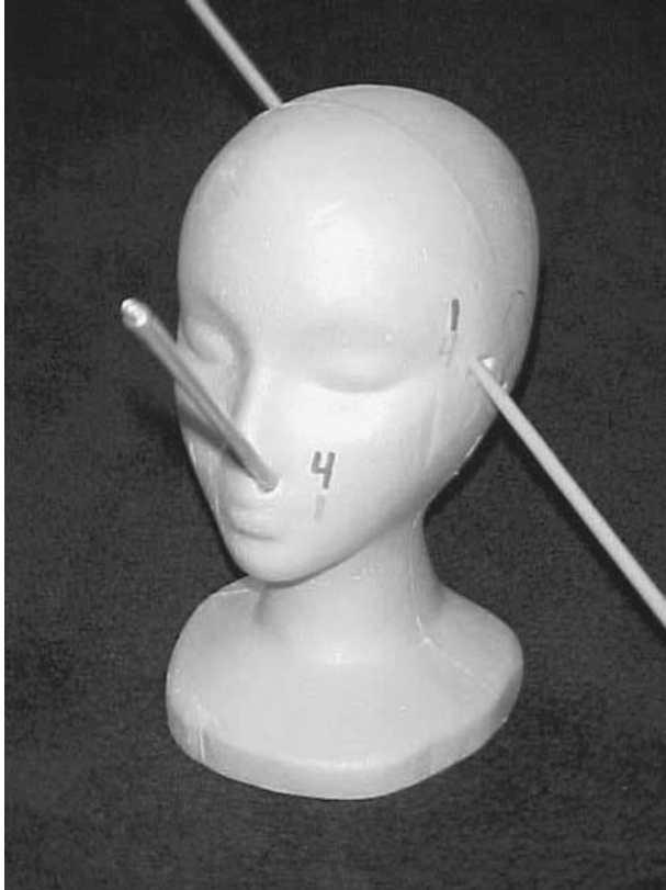
Figure 12.1 A Styrofoam head with trajectory rods used to help illustrate specific wounds and how they relate to the scene.
