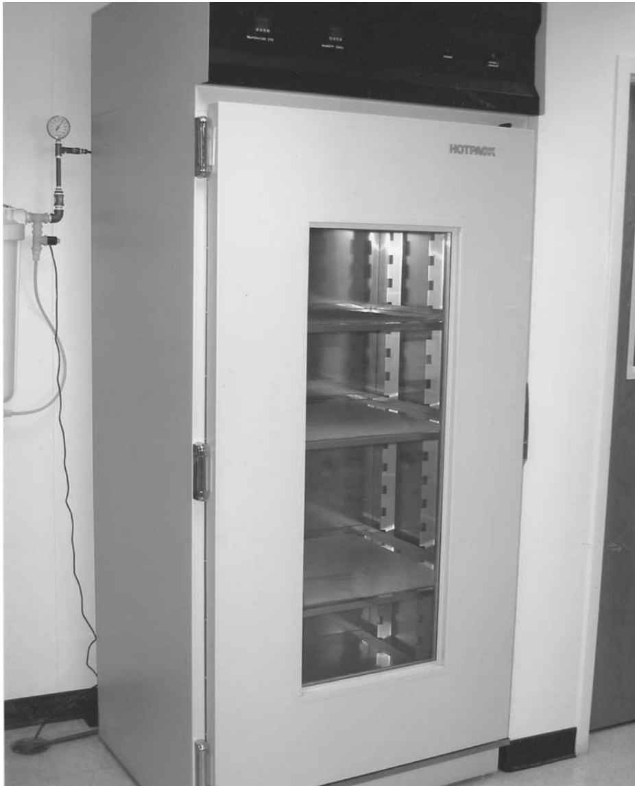
Figure 6.6 (A color version of this figure follows page 256.) Using a humidity cabinet speeds up the ninhydrin reaction to proteins found in fingerprints. ( Los Angeles County Sheriff's Department. )
