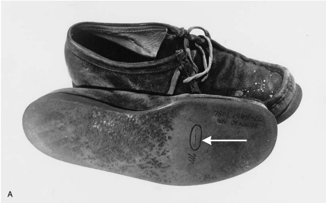
Figure 7.1 (A) Shoes seized from a breaking-and-entering suspect. Arrow indicates piece of glass in the crepe-rubber sole. (B) A close-up of the sole of the left shoe showing the piece of glass from the crime scene embedded in the tear. ( Royal Canadian Mounted Police, Forensic Laboratory Services. )
