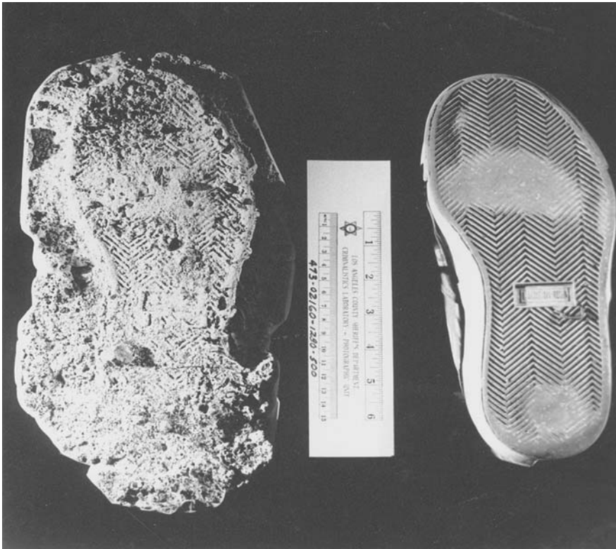
Figure 1.8 Sometimes class characteristics may be unusual enough to permit the inference that an item of evidence came from a single source. This illustration shows a plaster cast (left) taken from a burglary scene and the suspect's shoe (right). (The photographic negative was flipped in order to show the cast in reverse orientation so that the two items can be more easily examined.) The tread on the sole and that on the plaster cast have the same design and similar wear patterns. The staple in the sole, also found in the cast, is convincing evidence that this shoe made the impression. ( Los Angeles County Sheriff's Department. )
