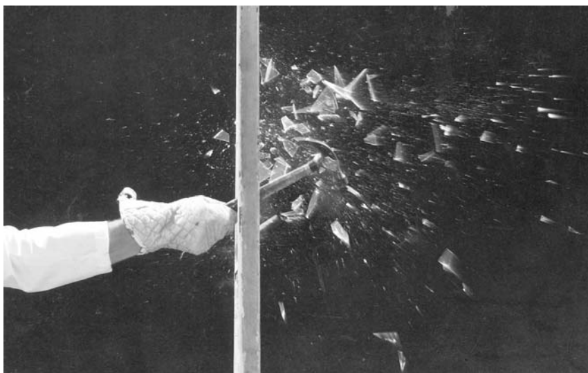
Figure 7.20 A burglar may be linked to a window he has smashed by the tiny fragments of glass that fly backward onto his person and clothing. ( Center of Forensic Sciences, Toronto. )
