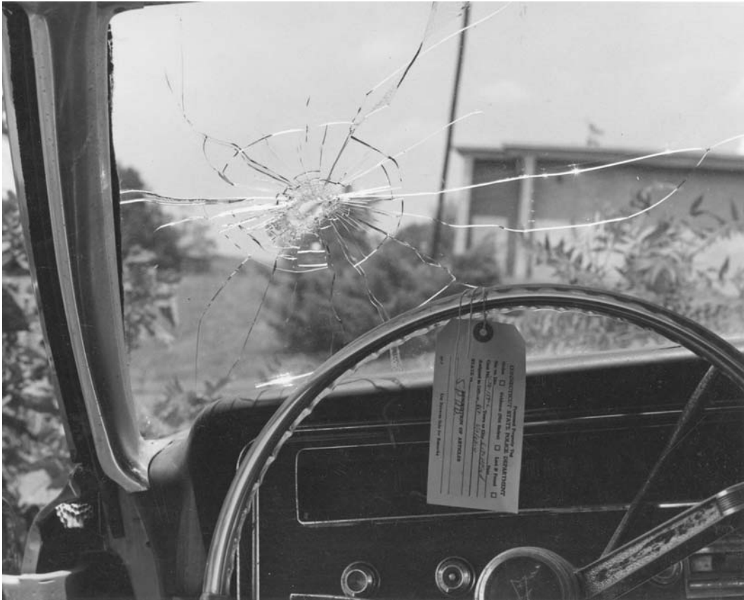
Figure 7.18 An actual case example of radial and concentric fractures in glass. ( Connecticut State Police. )
