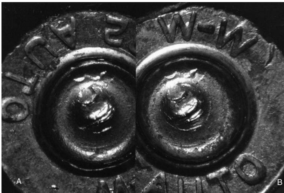
Figure 10.16 (A) Identification of a cartridge case of 7.65-mm caliber (.32 autos) with a suspect cartridge case (B). The microscopic details in the marks of the firing pin on the primer agree completely in the two cartridge cases. ( Los Angeles County Sheriff's Department. )
