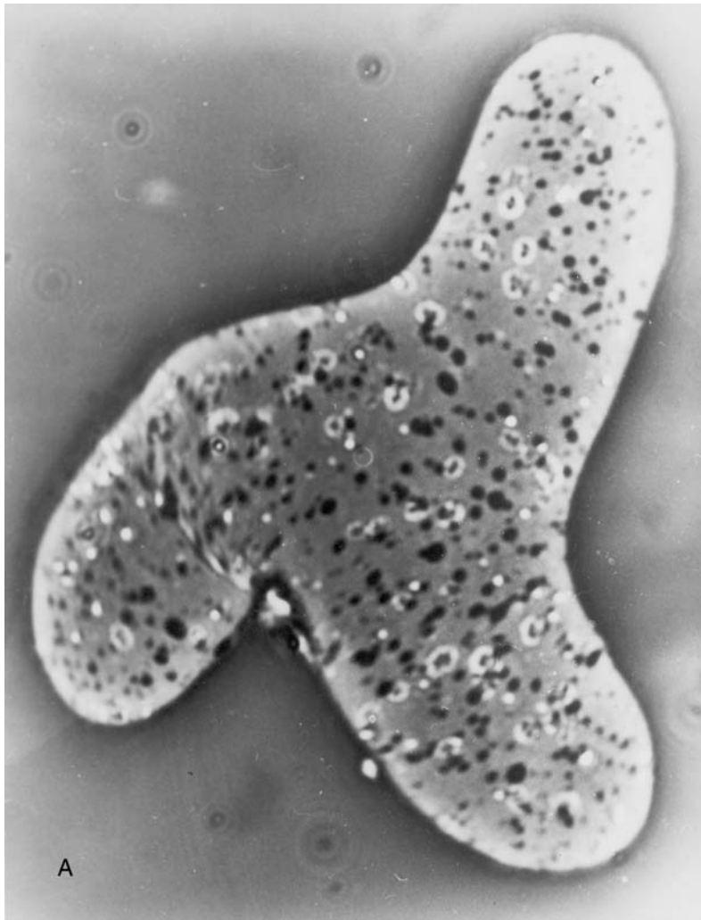
Figure 7.11 Fibers from one of the cases linked the victim to the assailants' home. A Monsanto Cadon® fiber (A) made only between 1968 and 1974 and a second rare modified "Y" fiber (B) produced by Rohm and Haas for a short period of time were important evidence in the trial. The defendants were found guilty of nine counts of murder and sentenced to life imprisonment without the possibility of parole. ( Los Angeles County Sheriff's Department. )
