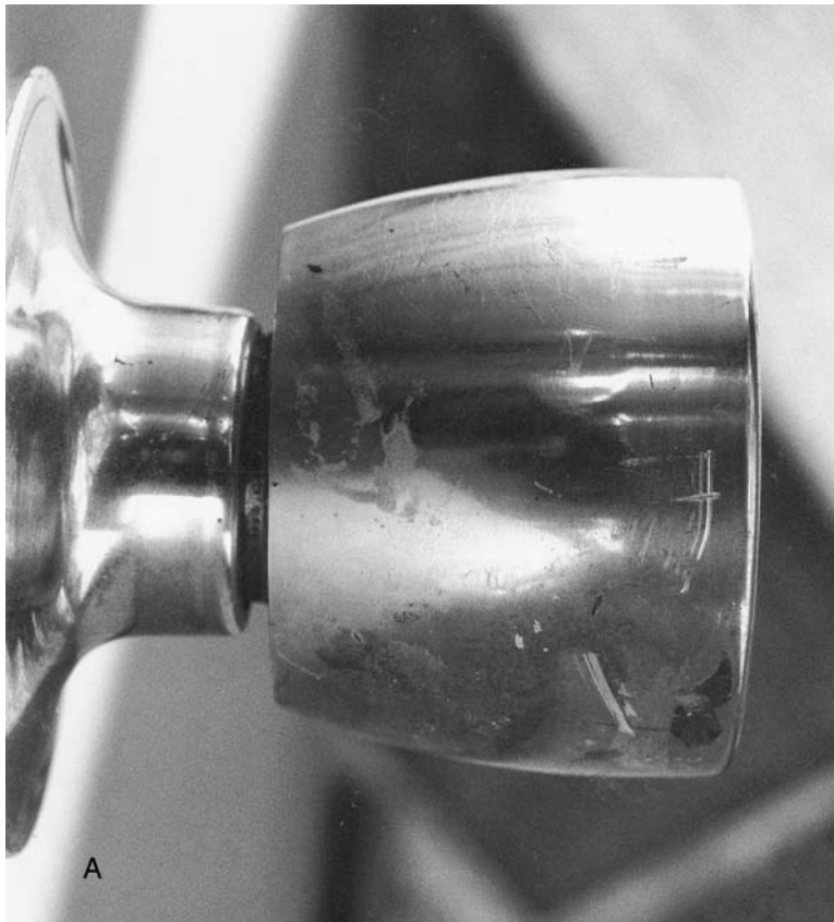
Figure 14.6 An exterior doorknob showing tool marks (A) and a pair of adjustable grips on a doorknob (B). Investigators should never attempt to match a tool to an object in this fashion. ( Los Angeles County Sheriff's Department. )
