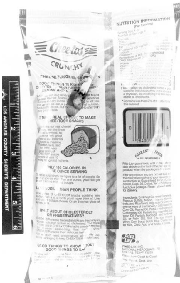
Figure 11.8 An improvised incendiary device consisting of a cigarette and matches can produce sufficient heat to cause the contents of the bag to burn. ( Los Angeles County Sheriff's Department. )
