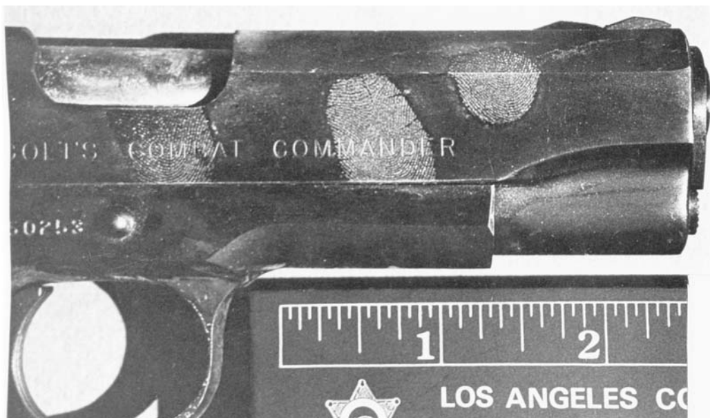
Figure 6.9 Latent prints developed using cyanoacrylate or superglue on a pistol. ( Los Angeles County Sheriff's Department. )
