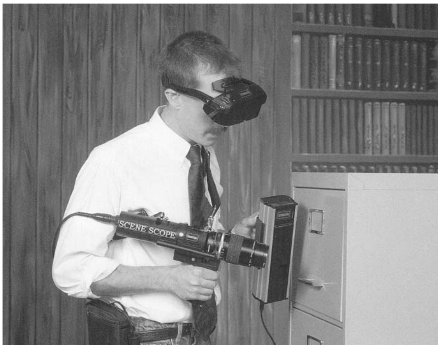
Figure 4.6 (A color version of this figure follows page 256.) New technology such as this SCENESCOPE® ultraviolet light imaging system can assist crime scene technicians to visualize trace evidence, such as latent prints that fluoresce under ultraviolet light. ( SPEX Forensics www.scenescope.com .)
