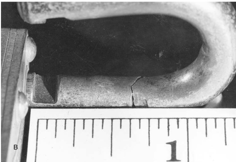
Figure 14.1 Evidence in a burglary case: (A) a cut lock hasp and (B) close-up of the hasp shown pieced together. ( Los Angeles County Sheriff's Department. )
