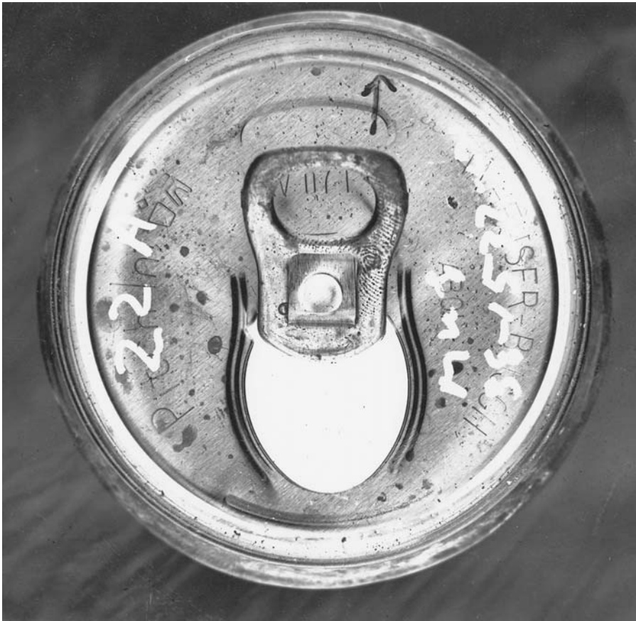
Figure 2.7 The suspect stated that he had never been in the murder victim's house in Ninilchik, Alaska. Trash from the victim's wastebaskets was examined for latent prints. A print was developed on the ring tab of a beer can using cyanoacrylate ester fuming. The latent print was compared to and identified with the suspect in the case. ( State of Alaska, Scientific Crime Detection Laboratory, Latent Print Section. )
