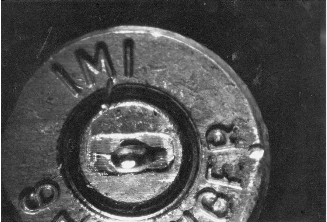
Figure 10.5 Determination of the make of pistol: cartridge case fired in the Austrian Glock 9-mm pistol; the rectangular firing pin hole is distinctive. ( Los Angeles County Sheriff's Department. )
