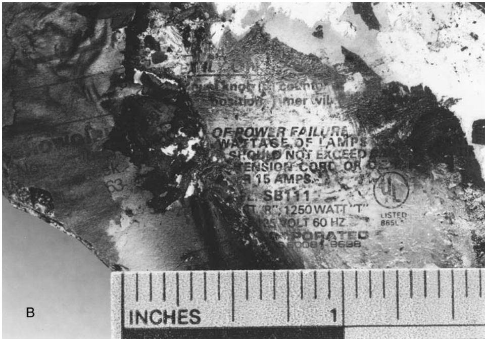
Figure 11.16 (A color version of this figure follows page 256.) A melted electrical timer device (A) and a close-up (B) showing a portion of a label believed to have been used in an arson case. The example of the intact timer (C) was used in the reconstruction of the device. ( Los Angeles County Sheriff's Department. )
