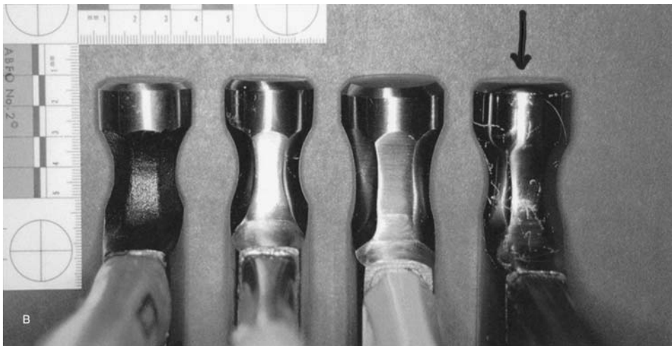
Figure 16.12 (A color version of this figure follows page 256.) Using a honeydew melon (A) to simulate a skull, tests with different hammers (B) suggested one that left a similar shape and dimensions in the victim's skull. ( Norman D. Sperber, DDS, San Diego, California. )
