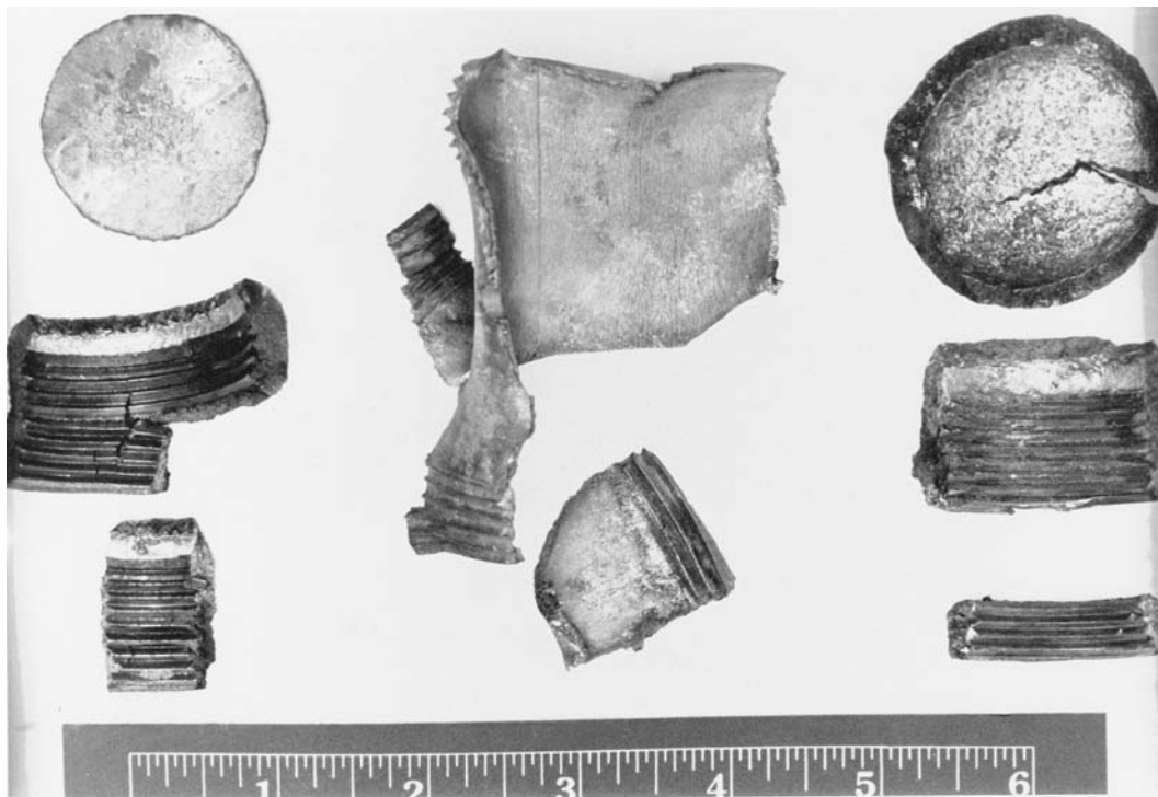
Figure 11.10 Debris from a pipe bomb packed with a low-order explosive. ( Los Angeles County Sheriff's Department. )
