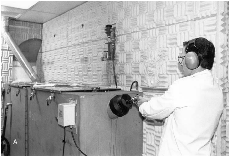
Figure 10.6 Weapons are test fired in a bullet recovery tank (A). The firearms identification expert makes use of a comparison microscope to compare bullets and cartridge cases (B). ( Los Angeles County Sheriff's Department. )
