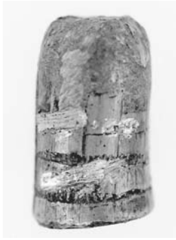
Figure 10.11 An evidence bullet carelessly marked in the region of the rifling impression. Valuable evidence was thereby destroyed. Bullets should be marked for identification on the base, and cartridge cases on the inside, near the mouth. However, a preferable procedure is to place the bullet in a container and label the package instead of the bullet. ( Los Angeles County Sheriff's Department. )
