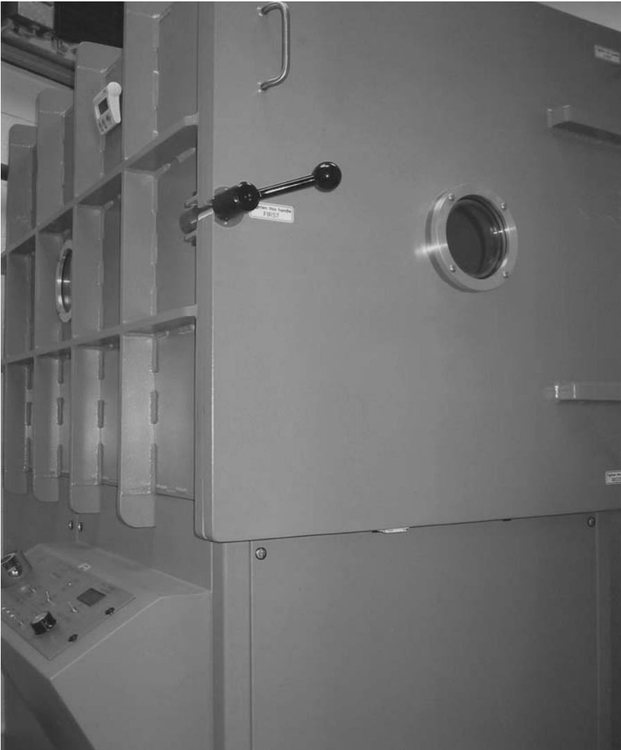
Figure 6.8 (A color version of this figure follows page 256.) The vacuum metal deposition places a thin film of gold followed by a film of zinc on latent prints left on smooth surfaces such as plastic bags. VMD is a very sensitive technique for fingerprint development on non-porous and semiporous surfaces. ( Los Angeles County Sheriff's Department. )
