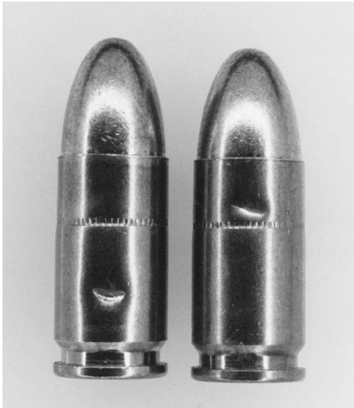
Figure 10.18 Automatic pistol cartridges (19-mm Luger) damaged by malfunctioning. The cases were jammed in the ejection port. ( Los Angeles County Sheriff's Department. )
