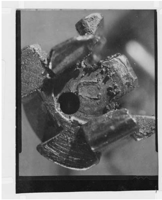
Figure 10.13 This figure illustrates a head stamp impression in the grease on a breechblock. (Contra Costa County Sheriff's Department, Criminalistics Laboratory, Martinez, California.)
