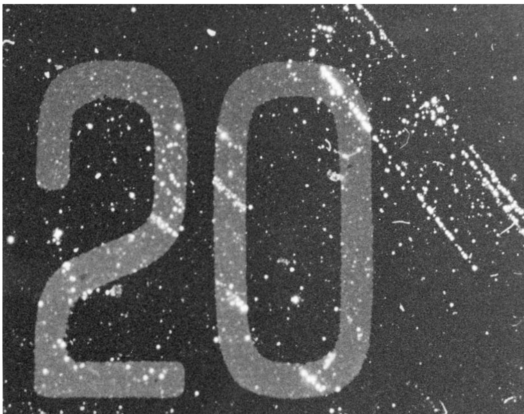
Figure 15.11 An investigator submitted a speedometer head to determine the speed of a vehicle at the time of impact. The speedometer dial was examined under ultraviolet light, and a “speed mark” was detected in the area of 20 MPH. This speed mark is an imprint of the speedometer pointer (needle) on the dial caused by the force of inertia at the time of impact. ( Forensic Laboratory, Office of Attorney General, Pierre, South Dakota. )
