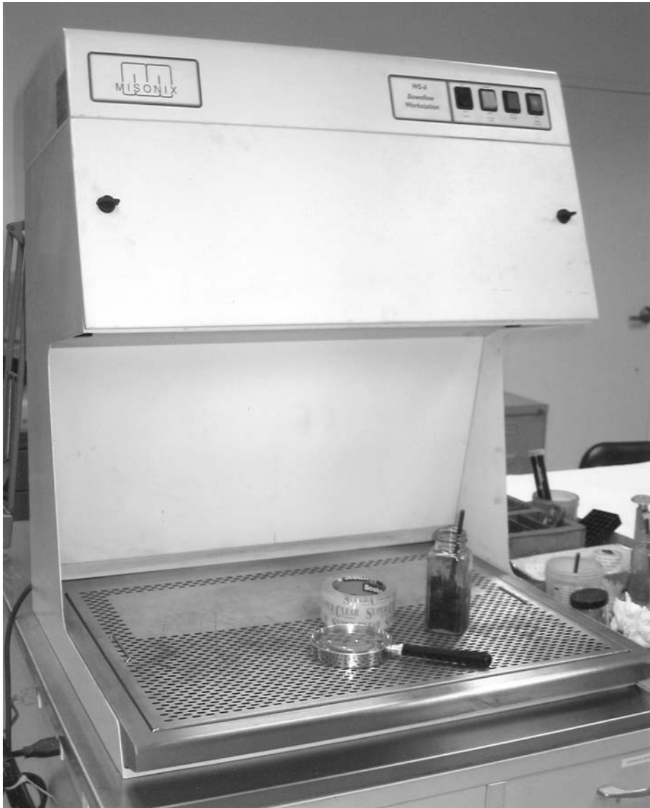
Figure 6.2 (A color version of this figure follows page 256.) Using a personal workstation with a ductless fume hood is an effective means to reduce the amount of fingerprint powder in the workplace. ( Los Angeles County Sheriff's Department. )
