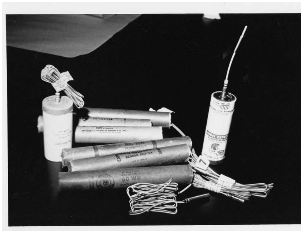
Figure 11.9 Examples of boosters, blasting caps, and dynamite. ( Los Angeles County Sheriff's Department. )
