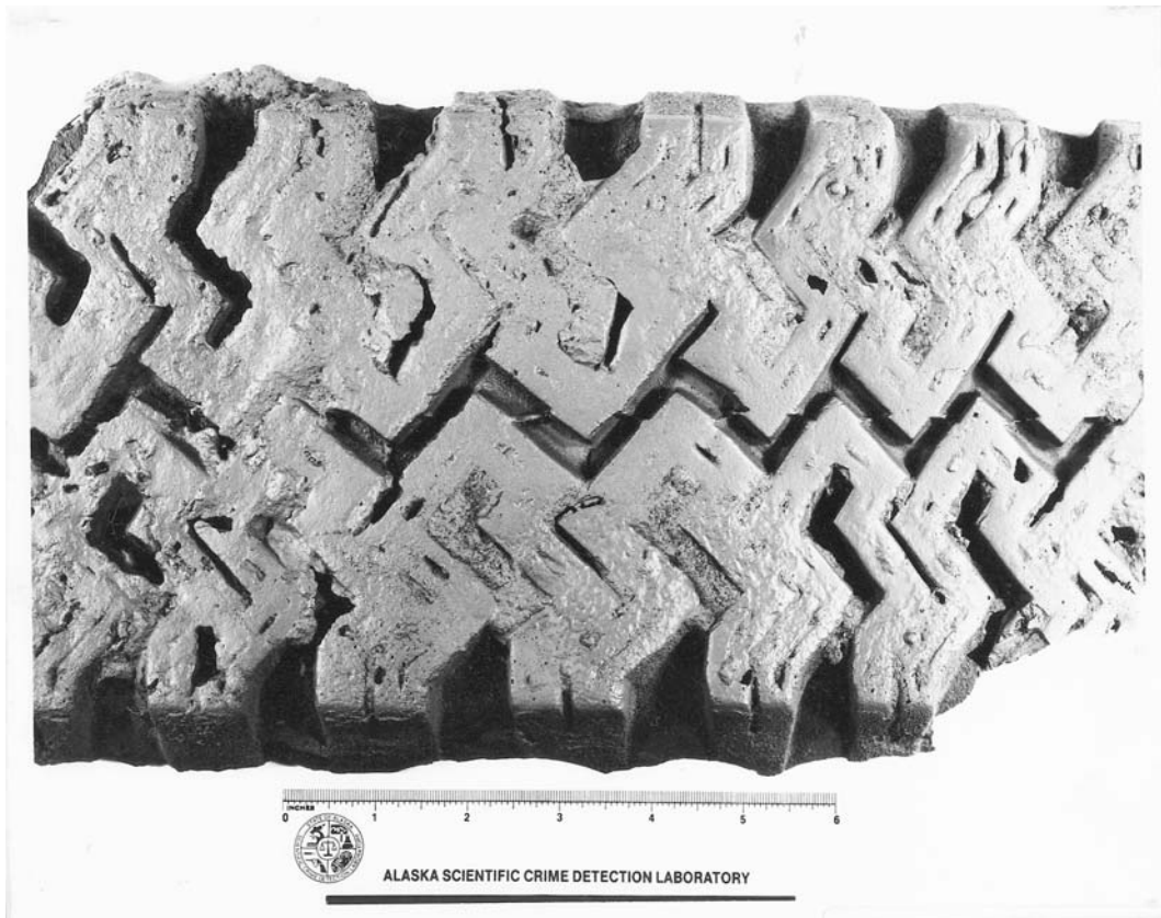
Figure 9.8 This dental stone tire casting was taken in a case involving the theft of several airplane propellers that was investigated by the Anchorage Airport Police. The tire impression was the first cast that the officer had ever poured in snow and enabled an easy identification because the tire had several bent studs. The technique used in Alaska in snow casting is to spray the impression first with gray automobile primer, which gives good contrast for photography and acts as a shell for the dental stone. The dental stone and water need to be ice cold prior to mixing. In extreme cold, potassium sulfate is added as an accelerator to the water and has been successfully used to cast impressions in conditions well below zero. ( Alaska Department of Public Safety, Scientific Crime Detection Laboratory. )
