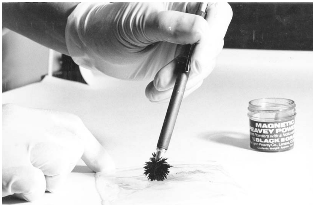
Figure 6.4 Magnetic fingerprint powders work well on some items. Only the rays of powder come in contact with the surface, as in this example on a plastic bag. ( Los Angeles County Sheriff's Department. )
