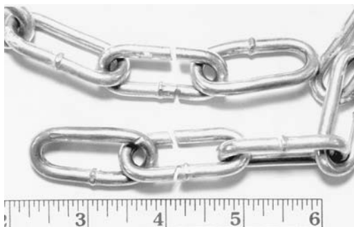
Figure 7.6 In the case of an alleged jailbreak attempt, the investigator wanted to know whether the inmate had used a hacksaw blade on his leg chains. When the crime was reenacted, a magnet was able to pick up numerous metal particles from the clothing of the investigator, whose hand was also slightly injured from using the blade. None of this evidence was found on the inmate, calling into question the hypothesis that he had tried to escape on his own. ( Los Angeles County Sheriff's Department. )
