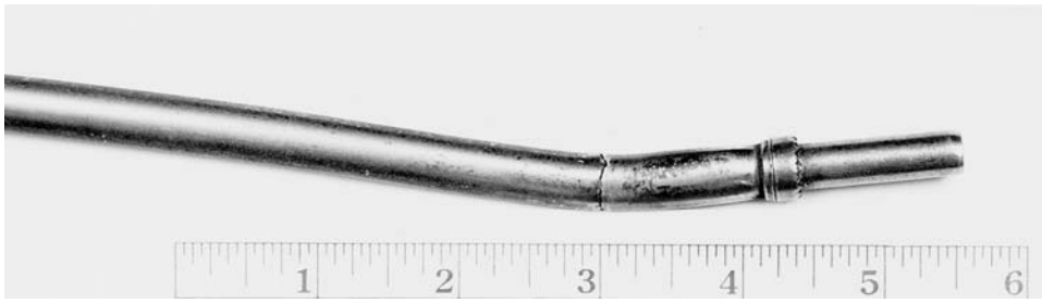
Figure 9.20 Physical match can be made on a wide variety of objects. In this case, pieces of a broken automobile antenna are shown pieced together. ( Los Angeles County Sheriff's Department. )
