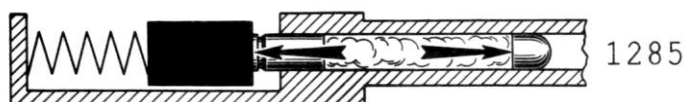
1285. The simplest form of operation—known as 'blowback'—is usually confined to guns chambering relatively weak cartridges. It relies simply on a heavy slide or breech block, a strong spring, and a stationary barrel. Blowback pistols are easy to make and effectual enough in their limited role.
