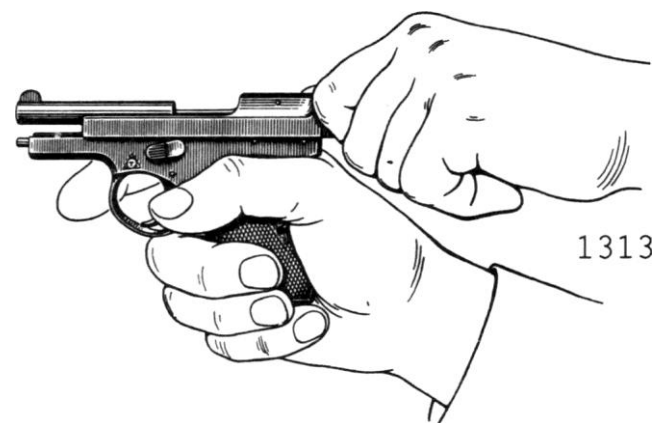
1313. Two hands are required to retract the slide of conventional guns—this is a Soviet 6.35mm TK—to chamber the round. Other forms of safety include trigger-locking buttons, catches to remove tension from the mainspring, bars which blocked the firing mechanism when the magazine was removed, and levers which could lower a cocked hammer safely onto a loaded chamber.
