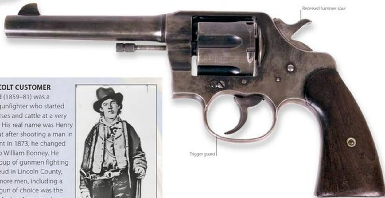
NEW DOUBLE-ACTION REVOLVER In the mid-1870s Colt finally began to make double-action pistols, starting with the "Lightning" model. The pistol shown here—which makes use of a slide-rod ejector to push spent cartridges from the cylinder chambers—is a model .38 made for export to Britain.
