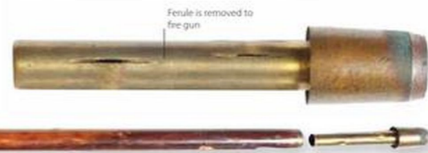
Brass top converts to a blowpipe
