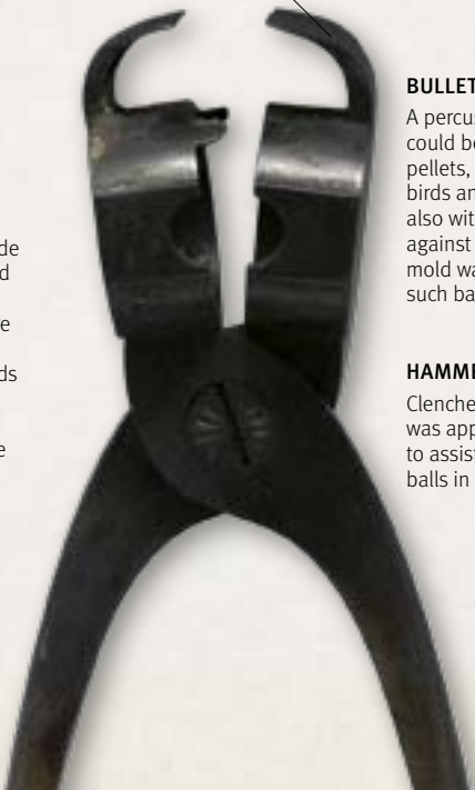
Cutters for removing flashing from moulded bullet
