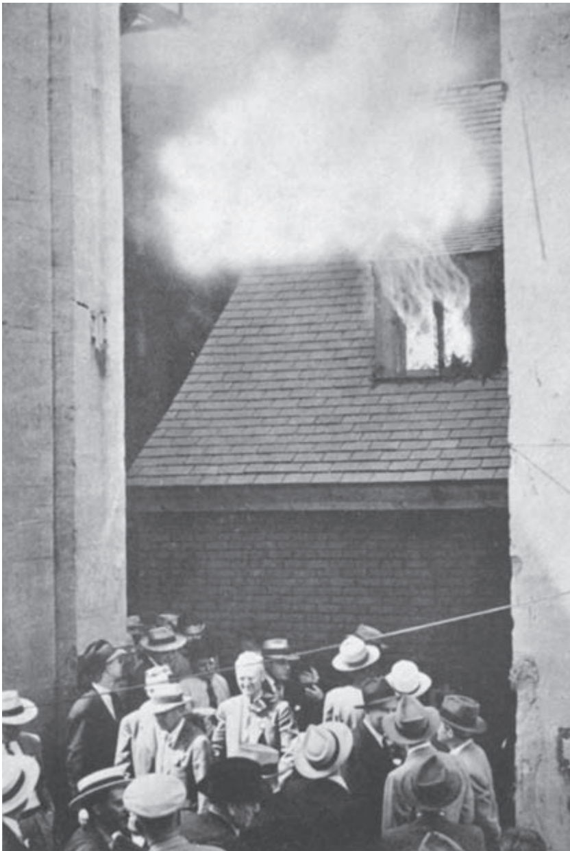
Flames pour from the second-story window of a test structure as spectators observe an incendiary bomb test by Standard Oil researchers in 1942–1943. Standard Oil Development Company/National Defense Research Committee
