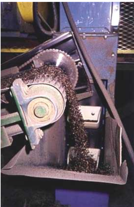
A conveyor belt drops a mixture of pure mânomin (black) and hulled mânomin (brown) into a “cup elevator.”
