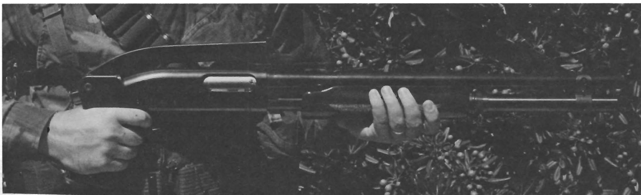
The Remington 870 "Brushmaster" 12-gauge shotgun, configured for combat. This version of the 870 is designed for rifled slugs and buckshot, and has adjustable rifle sights. Note the Choate folding stock, pistol grip, magazine extension, and sling. (Choate Machine and Tool Co., PO Box 218-FA Div., Bald Knob, Arkansas 72010.)
