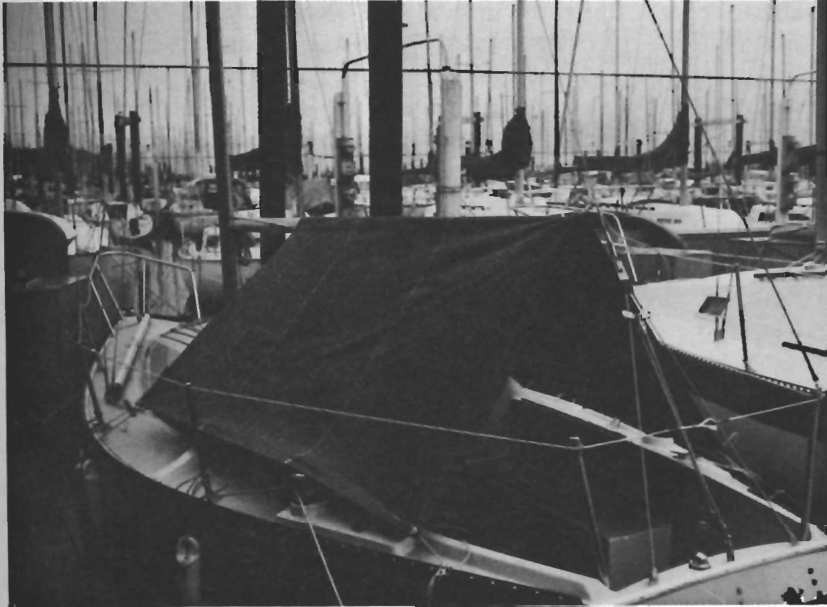
Sailboat equipped with a boom tent, the first essential piece of equipment in making a floating fallout shelter. (Tent courtesy of the Seattle Tent & Fabric Company, PO Box 33576, Seattle, Washington 98133.)
