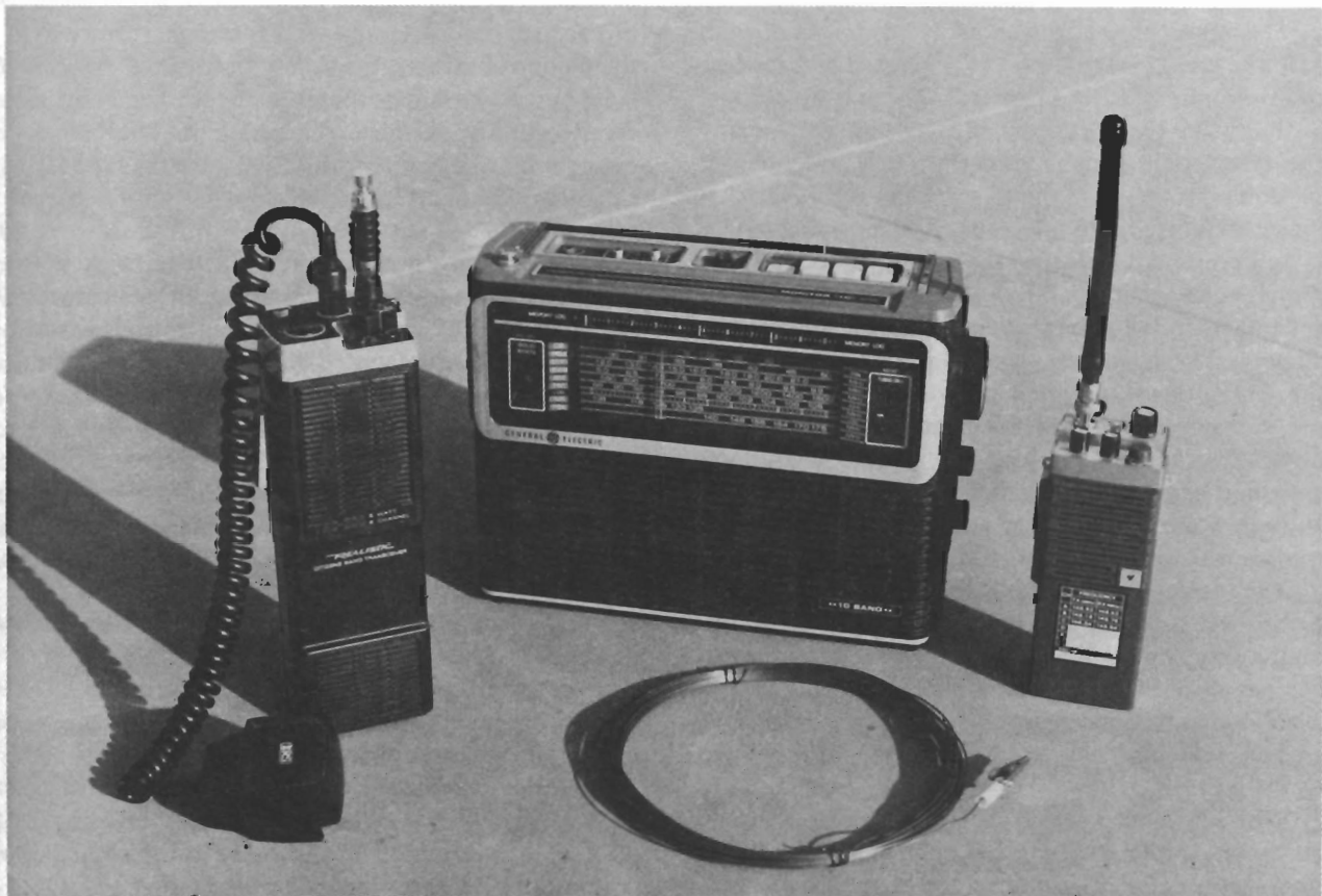
R adios of use to survivalists. Left, the Realistic 200 handi-talkie with its optional microphone (available from Radio Shack). Center, the General Electric ten-band portable. Right, a two-meter HAM unit made by Yaesu. Compared to the Realistic 200, the Yaesu has five times the battery life and ten times the range (used with a repeater station); the Yaesu has 800 channels. The roll of wire can be used as a makeshift antenna for the GE portable. (Yaesu unit courtesy of Harbor Electronic Marine Equipment Company (HEMEC), Santa Barbara, California.)
