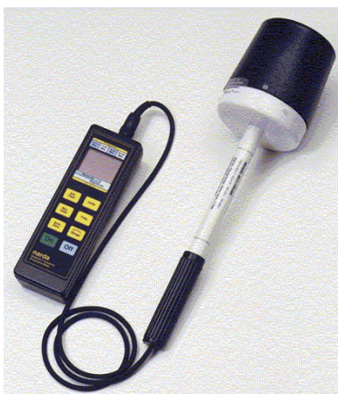
Figure 9-4. Modern Broadband RFR Survey Meter (courtesy of L-3 Communications, NARDA East).
