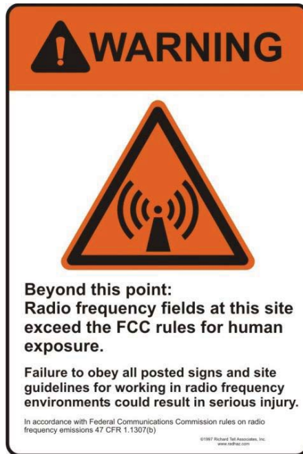
Figure 10-4. Example of an RF Warning sign following IEEE C95.2-1999.
