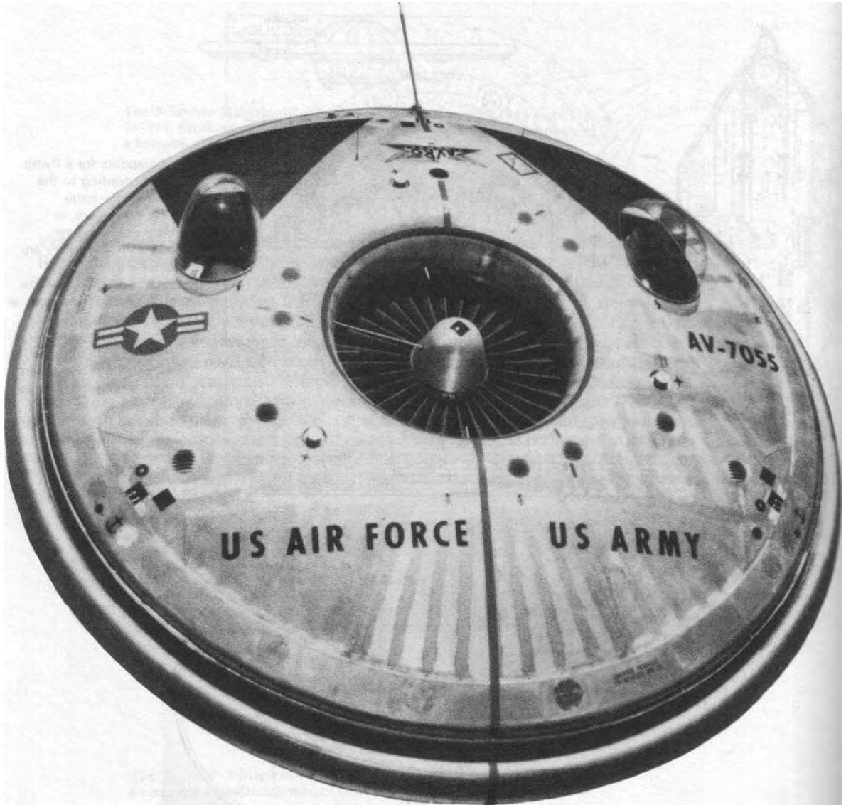
the Avro Car, built for the us Air Force and us Army by the Avro-Canada company. It was designed by an English engineer, John Frost. Officially, work on it was dropped in 1960 - despite the early claim that the machine would reach twice the speed of sound
