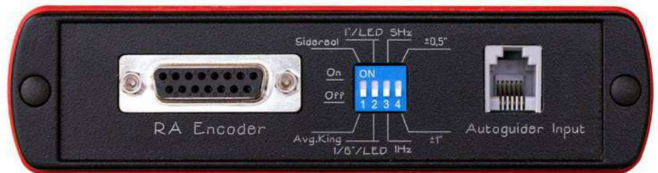
The Telescope Drive Master, from Hungarian company MDA-TelesCoop, is a novel way to correct periodic error, instantly improving the quality of your telescope's mount. ALL PHOTOS: MIKE REYNOLDS
