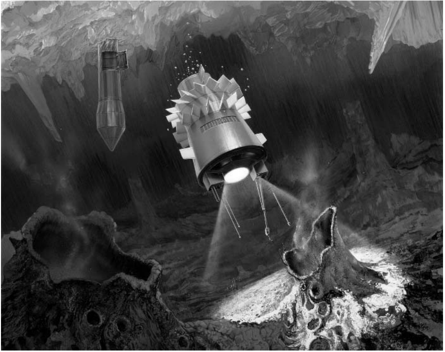
FIGURE 70 If there is an ocean beneath the ice of Europa, then a hydrobot similar to this artist's impression will probably be used to explore it. NASA scientists are currently examining the details of how to send a hydrobot to Europa, have it penetrate the ice and reach the ocean without introducing contamination, and then have it send back information to Earth.
