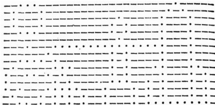
Figure 1b shows the same series of pulses arranged in the correct scanning pattern - with the horizontal rows containing twice those of the verticals - i.e., 30 x 15.
