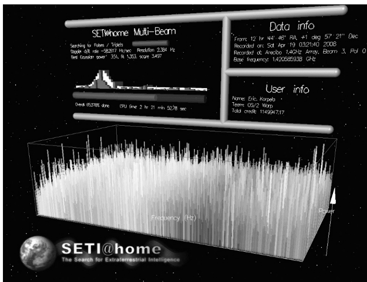
Figure 11.2 A screenshot of the SETI@home application graphical display. The bottom half of the screen presents the power spectrum currently being analyzed. The upper left section shows analysis state and the results of the current analysis. The upper right section shows information about the data being processed and the user's statistics.
