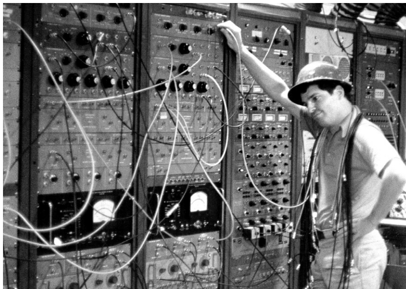
Figure 8.1 Paul Horowitz in the control room of the Arecibo Observatory, plugging together his first SETI receiver from the observatory's existing equipment.
