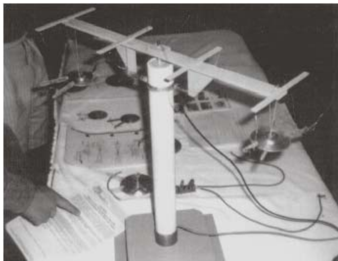
Figure 12.6. A small-size rotary electric disc setup built by Larry Deavenport to duplicate Thomas Townsend Brown's electrokinetic disc experiment. (Photo courtesy of L. Deavenport)
