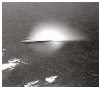
Figure 5.7. A B-2 bomber flying through humid coastal air at transonic speeds with a vapor cloud condensing behind its bow compression wave. (Photo by Bobbi Garcia, courtesy of the U.S. Air Force Flight Test Center)
