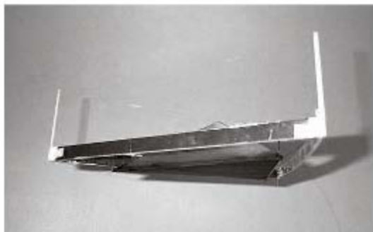
Figure 12.12. A lifter built and tested by Jean-Louis Naudin. (Photo courtesy of J.-L. Naudin, from his website, http://jnaudin.free.fr/ )
