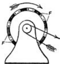
Figure 1.8. A gravitator motor composed of gravitator cells (F) positioned around the circumference of a wheel. (Brown, 1928)
