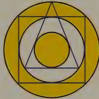
Figure 3-7. A derivative of Hawkins's second theorem? The central circle and the inner and outer edge of the surrounding ring include an isosceles triangle. Since the outer ring includes a square, this can only happen in one way, which defines the diameters of the ring and the circle, as well as the top angle of the triangle (slightly less than 46 degrees).
