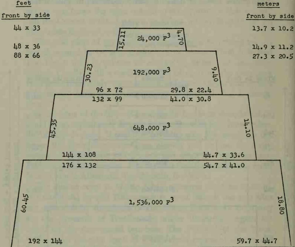
This drawing shows the original dimensions of the Ziggurat of Ur, in meters and in Sumerian feet of 0.310723 meters. It was built with 9.6 million bricks and its volume was 2.4 million cubic feet, or 720,000 cubic meters, which represented  $\frac{1}{6}$  of the volume of the Tower of Babel, or  $\frac{1}{36}$  of that of the Great Pyramid of Cheops. The first tier has a 132:144 ratio equal to 264:288.
