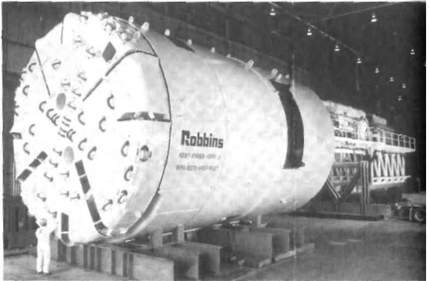
ILLUSTRATION 28 - Two tunnel boring machines (TBMs) sold by The Robbins Company. The top model was built for La Reunion irrigation project; the bottom one for Boston Outfall. The front ends of these TBMs chew away the rock; the structures that trail behind house the operators and carry away the muck. Photos used with permission from The Robbins Company.
