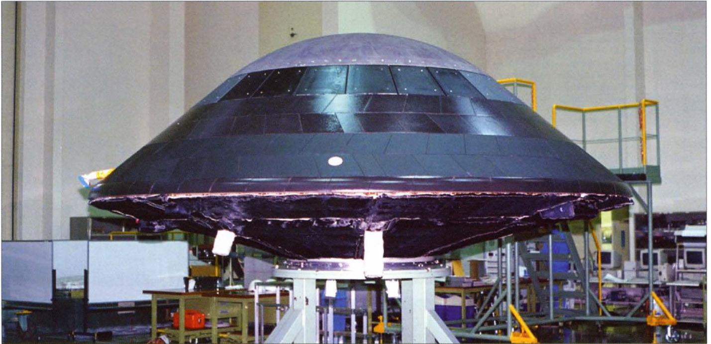
The Japanese designed and built Orex instrumentation capsule. Japan Aerospace Exploration Agency
