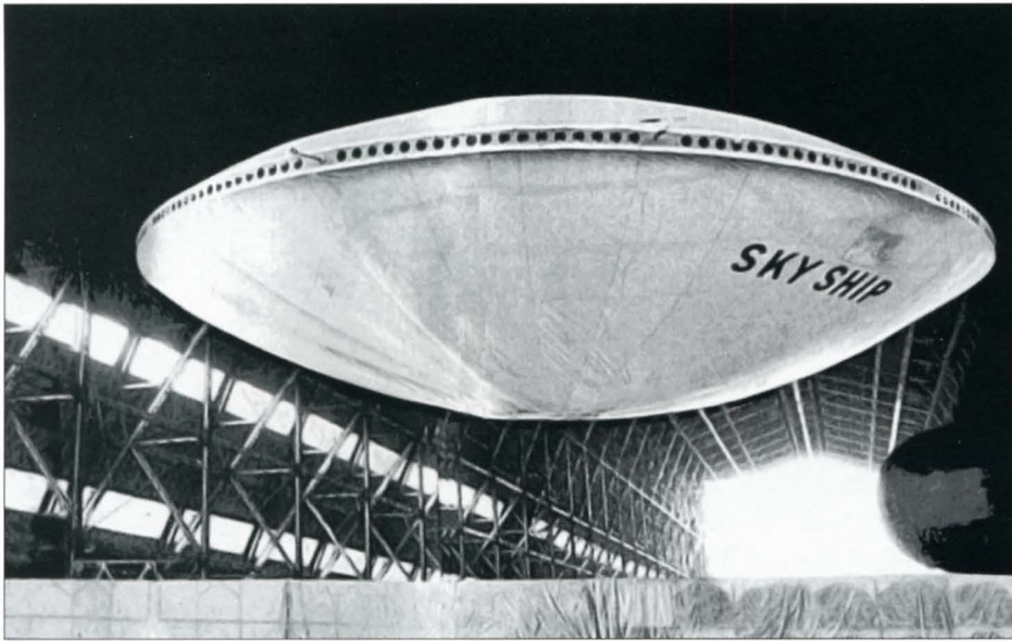
Skyship was a British flying saucer-shaped airship built at Cardington and completed during April 1975. Intended to be the scale prototype for a much larger series of vehicles, the project never advanced any further. via Bill Rose
