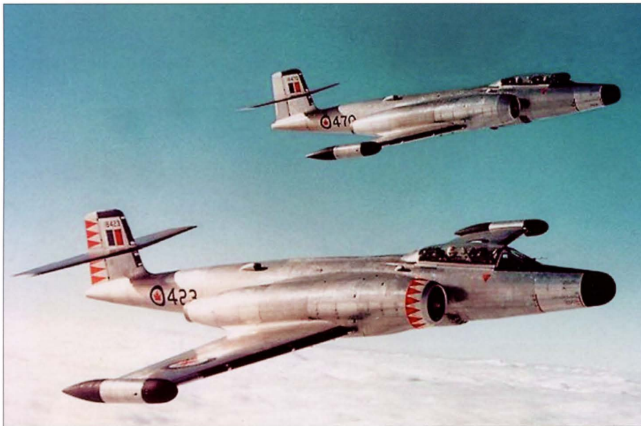
Left: Avro Canada CF-100 all-weather jet fighter. John Frost was recruited to head the design team for this aircraft in 1947. RCAF
