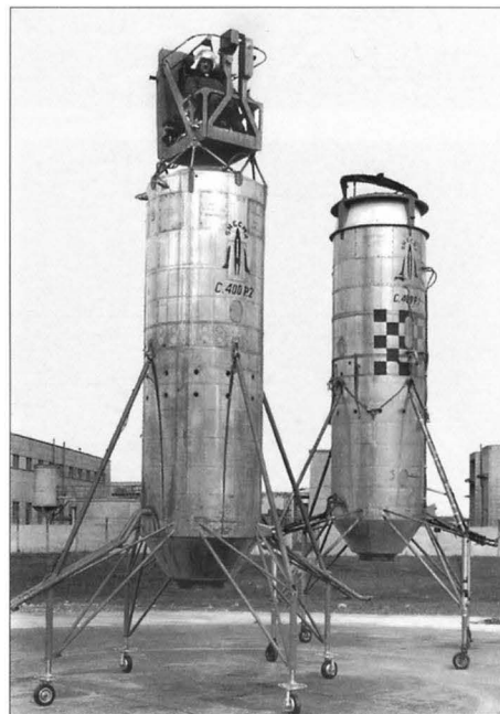
Above right: Produced in the early 1950s, this is an early SNECMA design for a VTOL jet fighter, which was clearly influenced by VTOL turboprop projects undertaken by Lockheed and Convair for the US Navy. SNECMA
