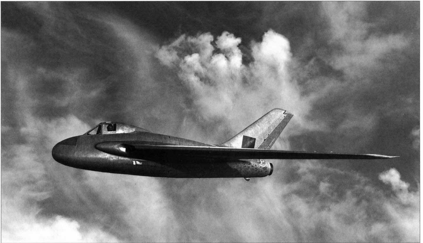
The second de Havilland DH.108 Swallow Experimental jet aircraft (TG306), which John Frost worked on before joining Avro Canada. The aircraft was destroyed in an accident over the Thames Estuary on 27th September 1946 when the airframe became structurally overloaded at a speed of about Mach 0.9, killing the test pilot Geoffrey de Havilland. de Havilland Aircraft Company, via Bill Rose
