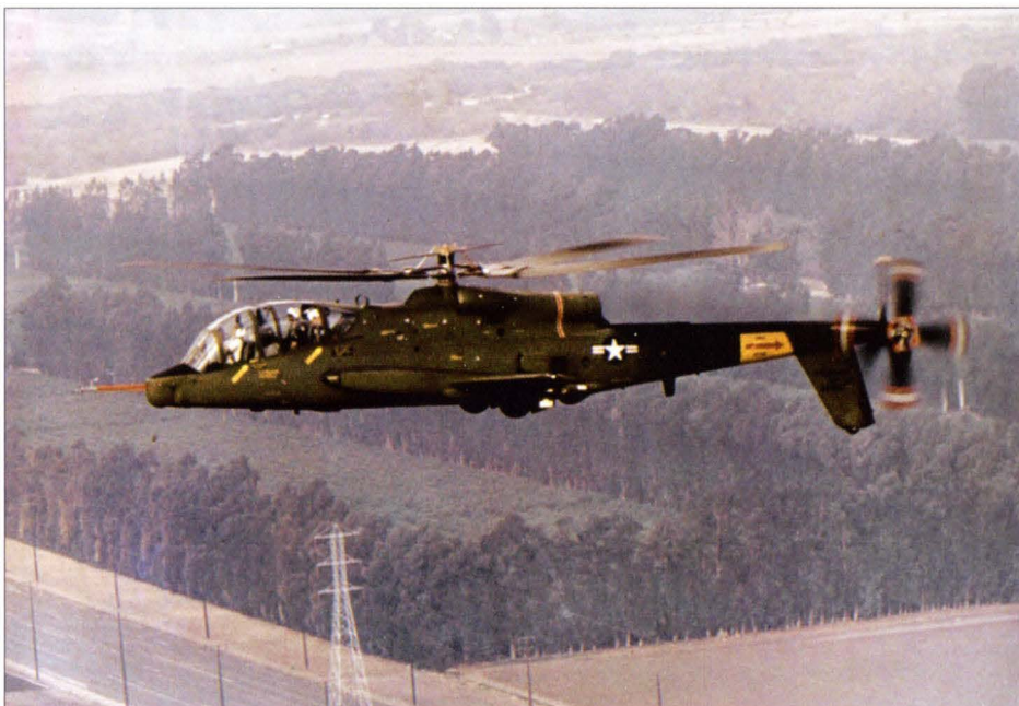
Lockheed AH-56 attack helicopter chosen as winner of the Advanced Aerial Fire Support System (AAFSS) competition in preference to the Convair Model 49. A small number of the aircraft were built and tested, but they were complex and expensive, so never entered production. However, the AAFSS eventually led to development of the Apache helicopter. US Army
