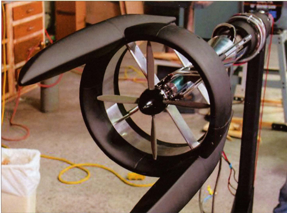
Above: Wind tunnel test model of the Honeywell Kestrel OAV, built by engineering subcontractor Techsburg. Techsburg
