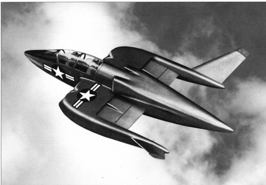
An early design study for the single-seat Vought ADAM demonstrator using a nose air intake. Ling-Temco-Vought
