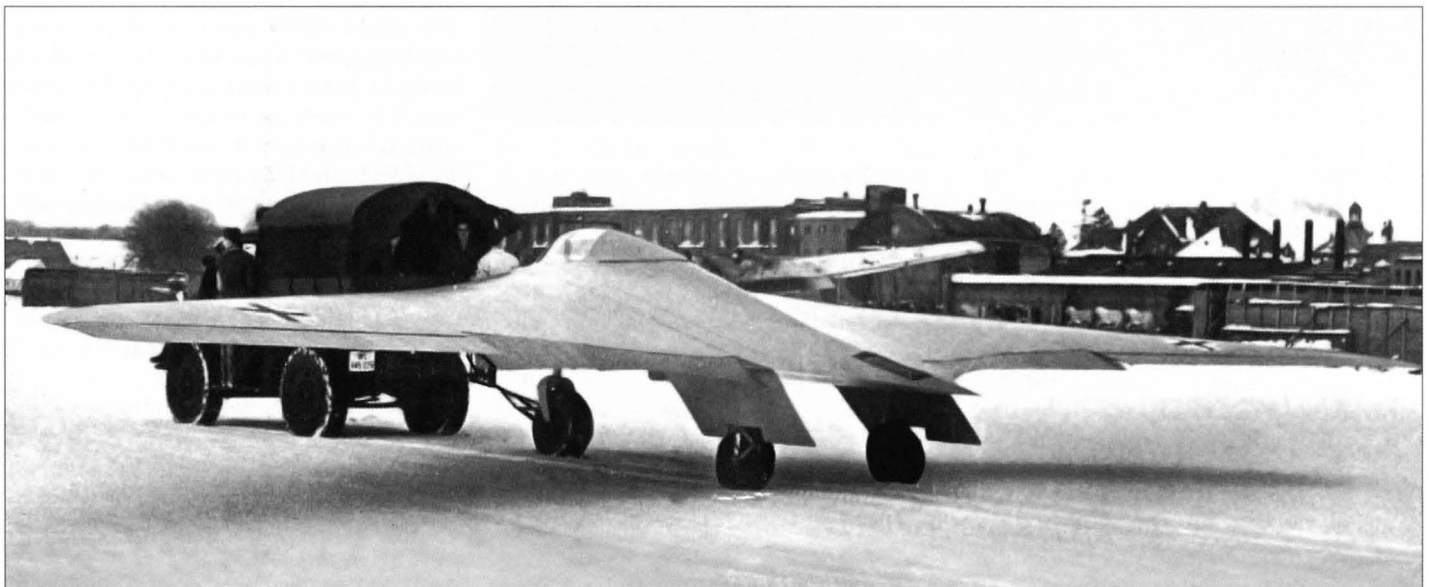
The Horten Ho 9 V1 is towed across a snow-covered airfield, probably in early 1944. Note the fixed rear wheels in streamlined fairings used on this initial prototype. After trials at Oranienburg, V-1 was moved to Brandis and finally destroyed by occupying US forces. Courtesy of David Myhra
