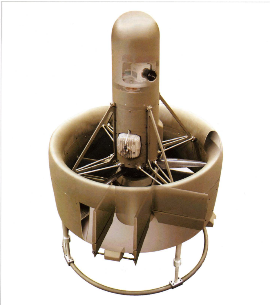
Above left: Honeywell ducted fan Class 1 OAV prototype. DARPA
