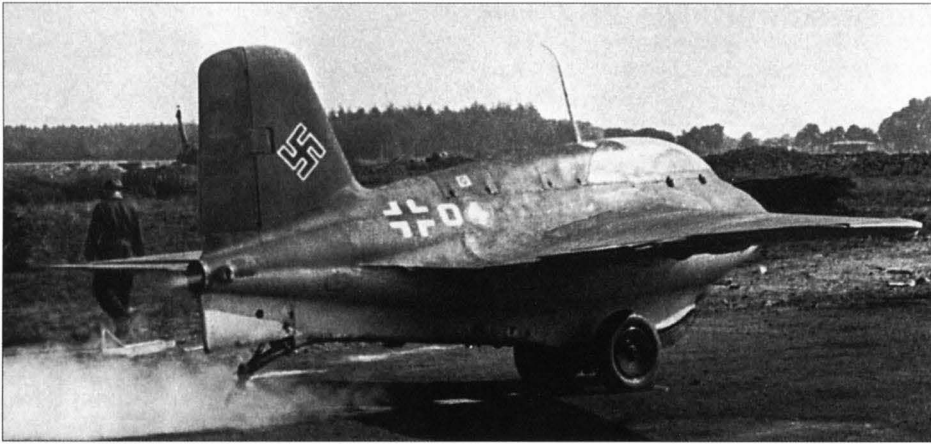
An Me 163B Komet begins a 'sharp' start in a cloud of steam, exhausted from a vent below the combustion chamber. Dangerous to operate and fly, the Me 163B was the fastest production aircraft of World War Two. via Bill Rose
