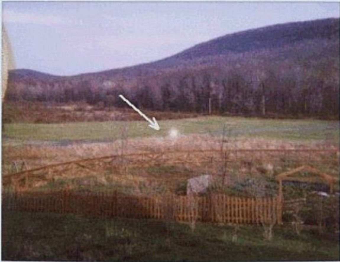
SUNLIGHT REFLECTED FROM A 1.25 INCH DIAMETER FRONT SURFACE ALUMINIZED MIRROR The mirror was about 280 ft from the camera.
