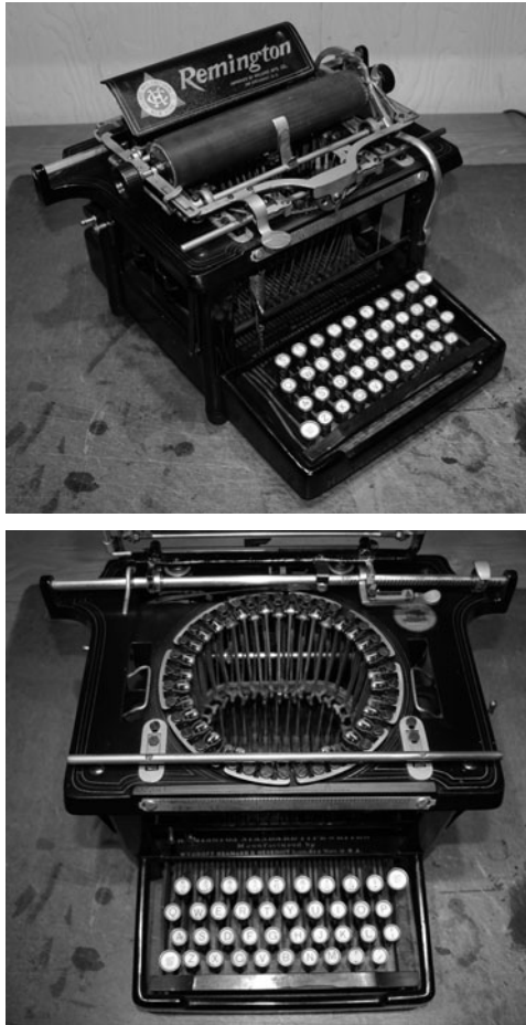
FIGURE 6.12 A Remington 2 typewriter from 1895, which was similar to its predecessor, the Sholes–Glidden Remington 1
