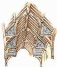
HAMMER-BEAM ROOF, CHURCH OF ST. BOTOLPH, TRUNCH, NORFOLK, BRITAIN, 1360-1380
