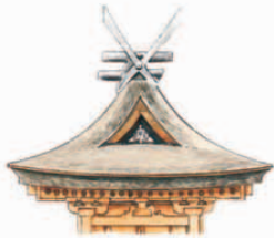
KASUGA-STYLE ROOF WITH SUMIGI (ANGLE-RAFTERS), KASUGADO SHRINE OF ENJOJI, NARA, JAPAN, 12TH-14TH CENTURY
