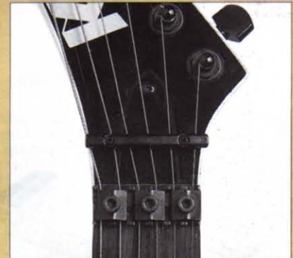
Locking nut (above) Strings are tuned approximately and locked using an allen key.
