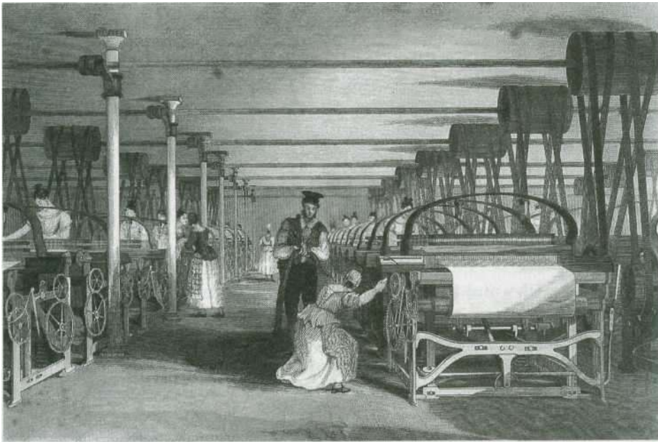
Power loom weaving in a cotton textile factory in 1834. Note that virtually all the workers are women.
