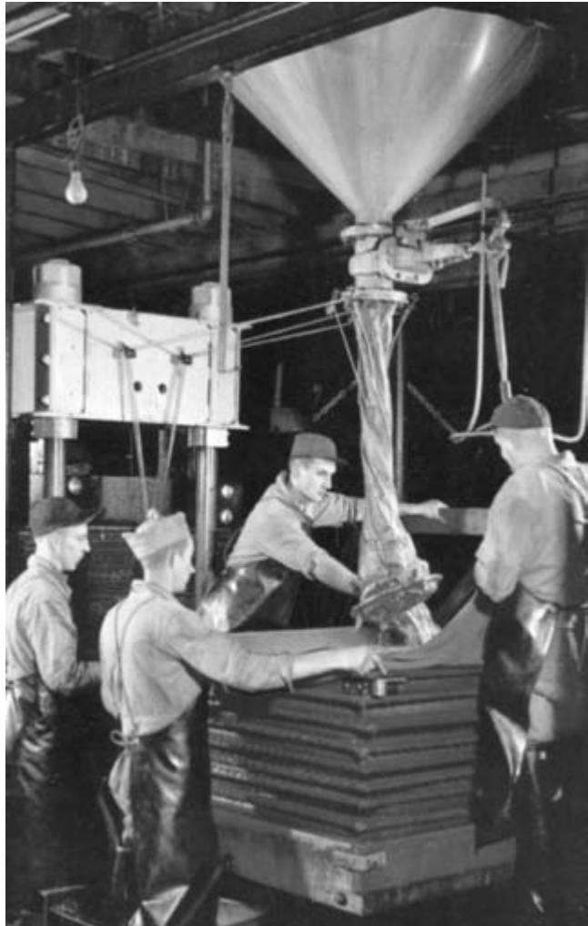
FIGURE 31 Loading a rack-and-cloth press at Pleasant Valley Wine Company of Hammondsport, New York. (Postcard in the author's collection.)
