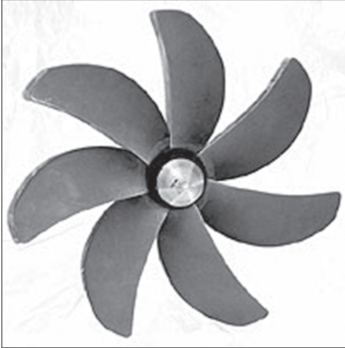
Figure 16.8. Because propeller design is so important to both speed and noise levels, it remains one of the most secret aspects of submarine technology. Used in design tests, this declassified model of the propeller from a 1960s Sturgeon-class fast attack submarine is the first ever put on public display.
