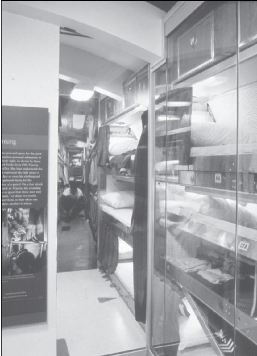
Figure 16.5. The personal space for the crew on a nuclear-powered submarine is extremely tight, as shown by these stacked bunks from the USS Trepang (SSN-674). The bins underneath the berths represent the only space a sailor has to store his clothing and other personal items for the duration of a patrol.
