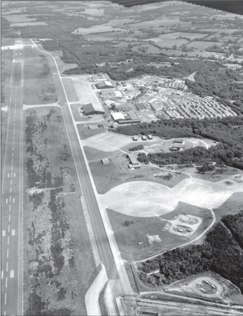
Figure 8.2. The Cold War runway, at 10,000 feet (3,048 metres), was one of the longest in Europe. This photograph, taken in 1995, shows the relationship of some elements of the base. The technical site (Area E) can be seen top right including the numerous barrack blocks for the bomber crews (laid out in curving streets to the extreme right). The Vehicle Maintenance, Wing HQ and Combat Support Buildings (Area D) are in the centre right and the northern fence of the GAMA complex (Area C) is located bottom right. The circular and diamond-shaped areas of hard standing were built in the 1950s to house bombers while on Reflex Alert. © English Heritage NMR 15288/36
